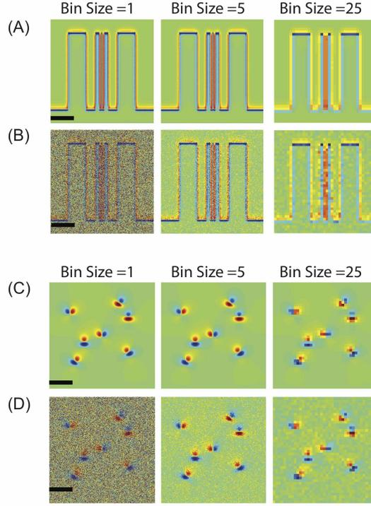
Figure 13: QDM Spatial Resolution and SNR Tradeoff. (A) Magnetic field from the current distribution in Fig. 4(A) for different planar binning sizes. No additional noise is applied. Scale bar is  $50 \mu\text{m}$  (B) Binning with fractional noise leading to SNR of 1 for a bin size of 1. (C) Magnetic field from magnetic dipole sources in Fig. 4(B). No additional noise is applied. Scale bar is  $10 \mu\text{m}$  (D) Binning with fractional noise leading to SNR of 1 for a bin size of 1.
