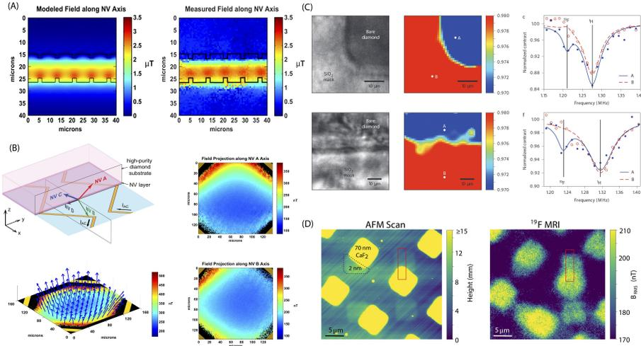
Figure 16: Examples of Low-Frequency QDM AC Magnetic Imaging. (A) Imaging magnetic field from current oscillating at 109.5 kHz [121]. (B) Imaging magnetic field from a wider field of view of current oscillating at 4.75 kHz [121]. (C) Imaging presence of  $^{19}\text{F}$  on diamond surface through NMR signal. Panel reprinted with permission from [122] (D) High spatial resolution imaging of patterned  $^{19}\text{F}$  on diamond surface [123]
