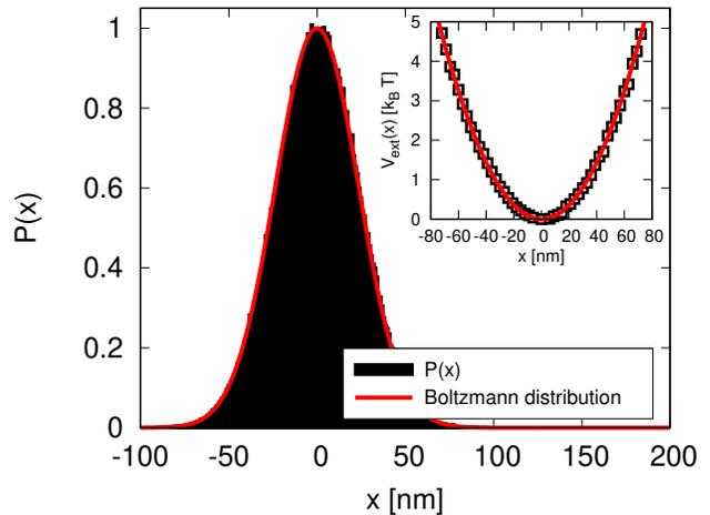
FIG. 2. Main graph: Probability distribution  $P(x)$  for a harmonically trapped particle, which is well described by the Boltzmann distribution shown as a red line. Inset: Measured trap potential (symbols) and a parabolic fit (solid line), from which the trap stiffness  $\kappa$  is extracted.
