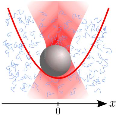
FIG. 1. Experimental setup of a colloidal particle in a micellar solution subjected to a harmonic confinement potential. The micrometer-sized particle performs a typical random walk in the limited configurational space in thermal equilibrium.
