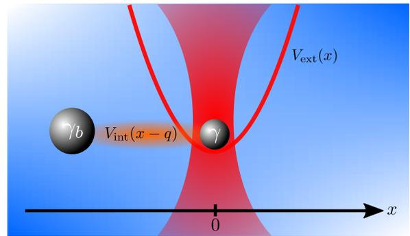
FIG. 4. Model of tracer and bath. The tracer particle (coordinate  $x$ ) is confined by a potential  $V_{\text{ext}}(x) = \frac{1}{2}\kappa x^2$ , tracer and bath are coupled via an interaction potential  $V_{\text{int}}(x-q)$ , where  $q$  is the coordinate of the bath particle.
