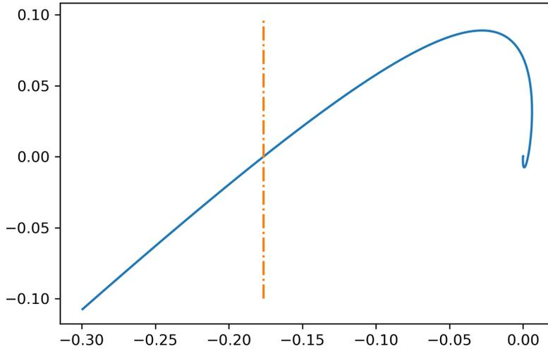
FIGURE 3. Popov plot  $P(G_{\text{loc}})$ . The limited resolution hides the infinitely many windings of the curve around the origin as  $\omega \rightarrow \infty$ .
