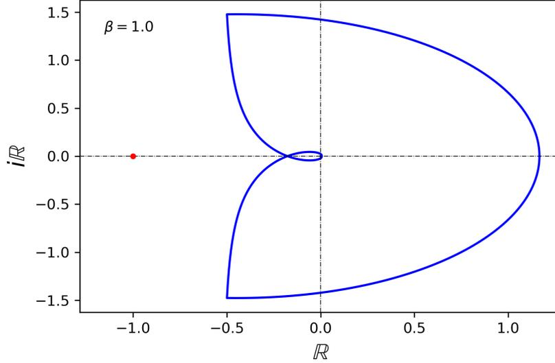
FIGURE 1. Nyquist plot  $\text{Nyquist}(G_{\text{nloc}})$ . The limited resolution hides the infinitely many windings of the curve around the origin as  $\omega \rightarrow \pm\infty$ .
