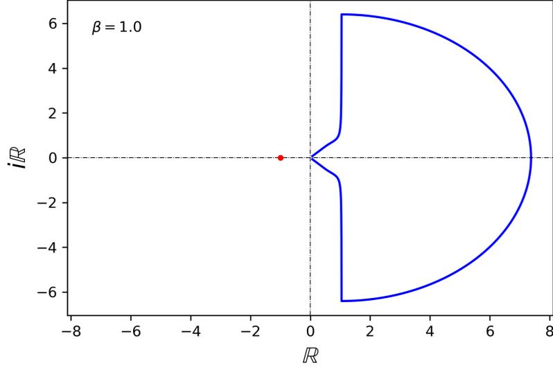
FIGURE 2. Nyquist plot of the transfer function  $G_{\text{loc}}$ .
