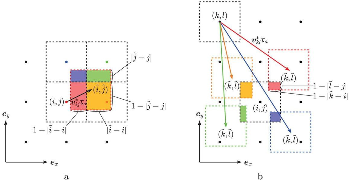
Figure 7: Advection in the particle picture. (a) Advection from the cell at lattice point  $ij$ . (b) Advection from the cell at lattice point  $kl$  to the cell at lattice point  $ij$ .
