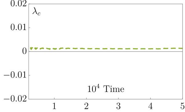
Figure 27: Conditional Lyapunov exponent  $\lambda_c$  for the synchronized chaotic attractor right after it comes to exist at  $\delta = 0.106, W = 0.055$ . A positive  $\lambda_c$  demonstrates the unstable nature of the attractor. Contrast this with Fig. 25, where the synchronized chaotic attractor at  $\delta = 0.080, W = 0.055$  is stable and hence leads to  $\lambda_c < 0$ .
