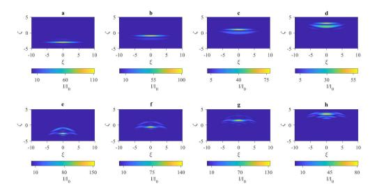
Fig. 2. Distribution of the quantity  $I/I_0 = (\partial \Psi/\partial \tau)^2$  in an array of nanotubes at various instants of dimensionless time  $\tau$  during the passage of the wave packet, which is the solution of Eq. (5): (a)  $\tau = 0$ , (b)  $\tau = 2.0$ , (c)  $\tau = 4.0$ , (d)  $\tau = 6.0$ , (e)  $\tau = 28.0$ , (f)  $\tau = 30.0$ , (g)  $\tau = 32.0$ , (h)  $\tau = 34.0$ .
