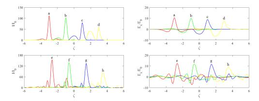
Fig. 3. Distribution of the electric field strength  $E_x/E_0$  and energy intensity  $I/I_0$  on the  $\zeta$ -axis, in the course of the propagation of the electromagnetic pulse shown in Fig. 2, at various instants of dimensionless time: (a)  $\tau = 0$ , (b)  $\tau = 2.0$ , (c)  $\tau = 4.0$ , (d)  $\tau = 6.0$ , (e)  $\tau = 28.0$ , (f)  $\tau = 30.0$ , (g)  $\tau = 32.0$ , (h)  $\tau = 34.0$ .
