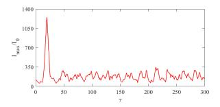
Fig. 4. Dependency of the ratio  $I_{\rm max}/I_0$  on the dimensionless time  $\tau$  during the propagation of the electromagnetic pulse shown in Figs. 2 and 3. The dimensionless time  $\tau=\omega_0 t/\sqrt{\varepsilon}$  is plotted along the horizontal axis.
