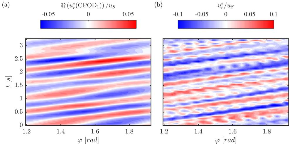
FIGURE 20. Space-time diagram of (a) the reconstructed radial velocity component based on the first CPOD mode and (b) the full field radial velocity component for  $Re_S = 9.32 \times 10^3$  and  $\mu = 0$  ( $C_1$ ) at the axial height of the vortex center as function of  $\varphi$  and  $t$ . The radial coordinate is fixed at  $\tilde{r} = 0.5$ .
