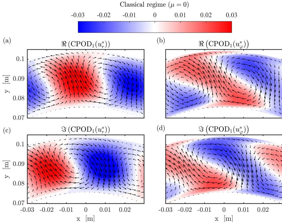
FIGURE 18.  $\mathbf{CPOD}_1$  for  $Re_S = 9.32 \times 10^3$  and  $\mu = 0$  ( $C_1$ ) at the axial height of the vortex center for both velocity components. (a) Real and (c) imaginary part of  $\mathbf{CPOD}_1$  for the radial velocity component. (b) Real and (d) imaginary part of  $\mathbf{CPOD}_1$  for the azimuthal velocity component. Black arrows represent the resulting velocity field of  $\mathbf{CPOD}_1$ .
