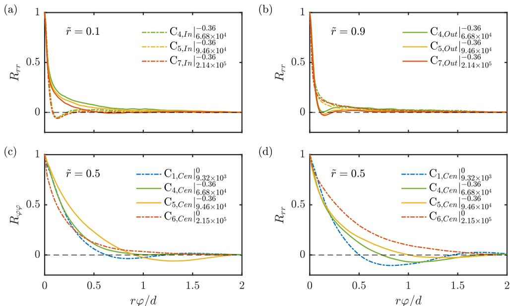
FIGURE 17. Upper row: Azimuthal two-point autocorrelation function of the fluctuation radial velocity component at the axial height of vortex in- and outflow at (a)  $\tilde{r} = 0.1$  and (b)  $\tilde{r} = 0.9$ . Lower row: Azimuthal two-point autocorrelation function of the fluctuation (c) azimuthal and (d) radial velocity component at the axial height of vortex center at  $\tilde{r} = 0.5$ . Legend abbreviations represent  $C_{\#}|\mu_{ReS}$ .
