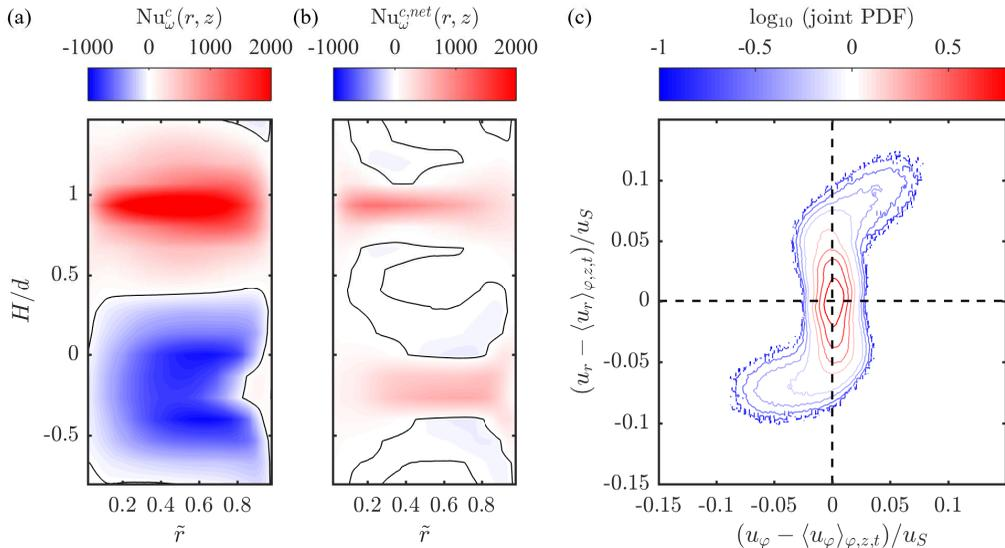
FIGURE 10. Contour plot of the dimensionless (a) convective and (b) net convective local angular momentum transport in a meridional plane for  $Re_S = 2.14 \times 10^5$  and  $\mu = -0.36$  ( $C_7$ ). Black lines indicate the zero line of the depicted quantities. The color codes are given in the legends. (c) Joint PDF of the radial and azimuthal velocity fluctuations for the same flow state at  $\tilde{r} = 0.5$ . The colors give the probability (in log-scale), see legend.
