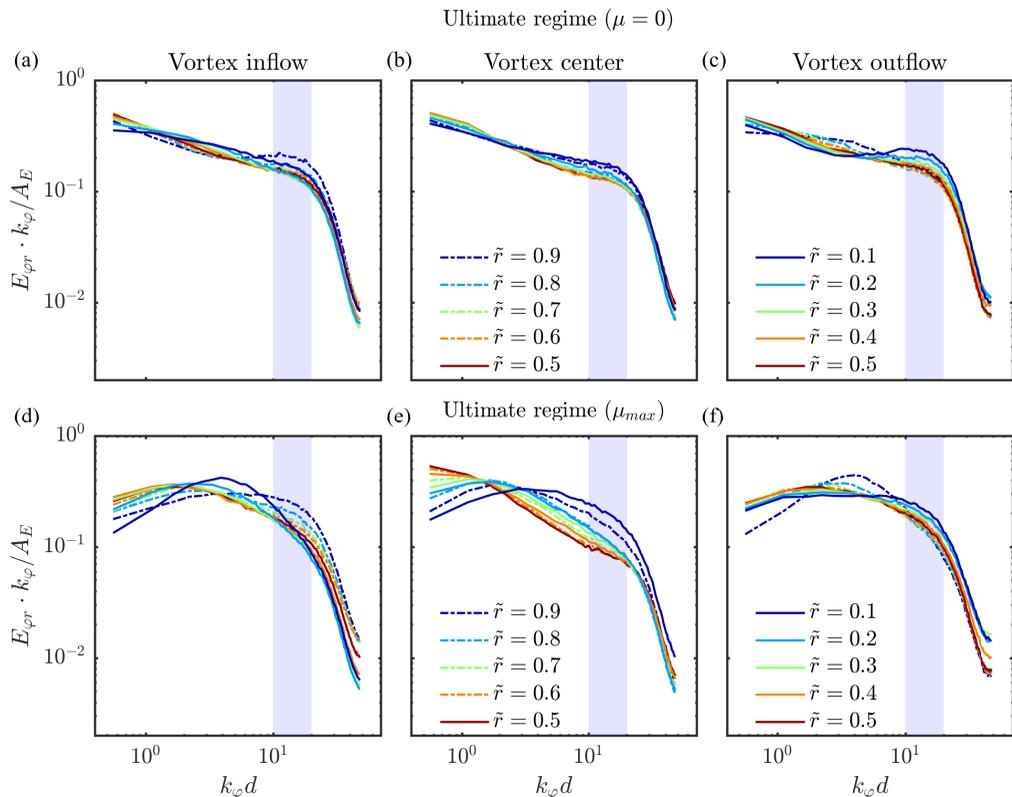
FIGURE 16. Upper row: Temporally averaged pre-multiplied azimuthal kinetic energy co-spectra for  $Re_S = 2.15 \times 10^5$  and  $\mu = 0$  ( $C_6$ ) at different radial positions at the axial height of (a) vortex inflow, (b) vortex center and (c) vortex outflow. Region of  $k_{\varphi} d \in [10, 20]$  is marked in light blue. Lower row: Same spectra for  $Re_S = 2.14 \times 10^5$  and  $\mu = -0.36$  ( $C_7$ ) at the axial height of (d) vortex inflow, (e) vortex center and (f) vortex outflow.
