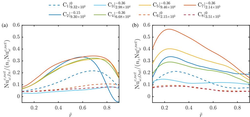
FIGURE 11. Radial profiles of the contribution of the net convective momentum transport of the (a) inflow and (b) outflow to the total transport.  $n_z$  represents the number of heights included into the average over cylindrical surfaces. Legend abbreviations represent  $C_{\#}|_{Re_S}^{\mu}$ .
