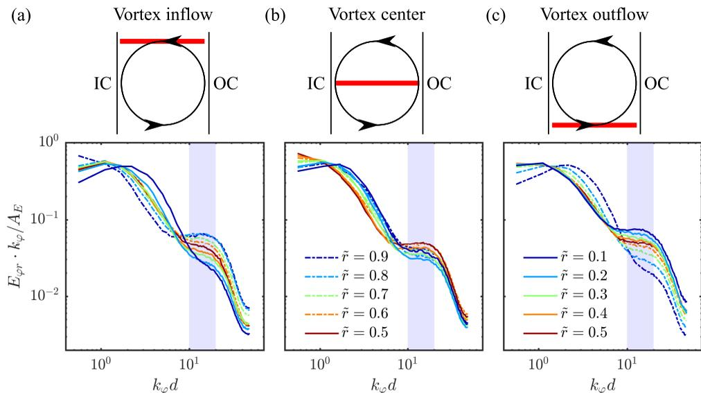
FIGURE 15. Temporally averaged pre-multiplied azimuthal kinetic energy co-spectra in the classical regime for  $Re_S = 9.30 \times 10^3$  and  $\mu = -0.15$  ( $C_2$ ) at different radial positions at the axial height of (a) vortex inflow, (b) vortex center and (c) vortex outflow. The region of  $k_{\varphi} d \in [10, 20]$  with enhanced plume emission is marked in light blue. Sketches above the co-spectra for the different vortex regions are added for clarity.
