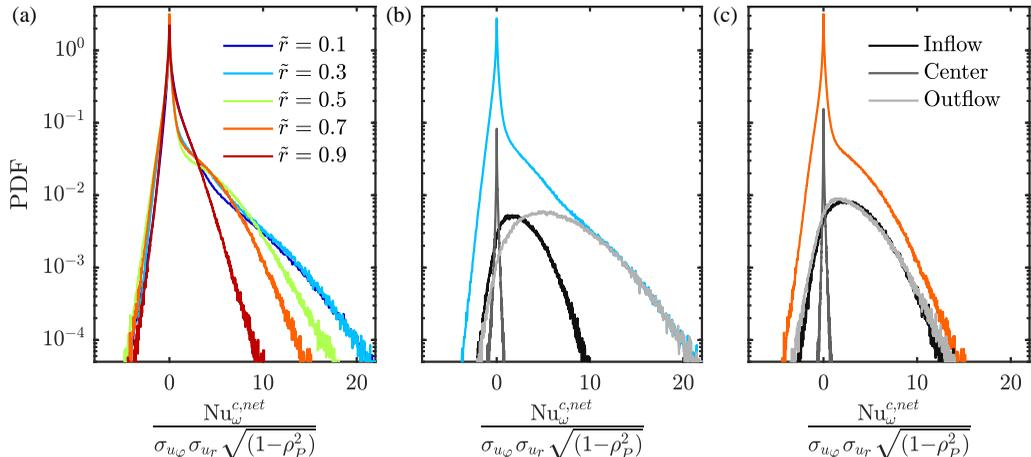
FIGURE 13. (a) Probability density functions of the local net convective angular momentum transport calculated over space (cylindrical surfaces) and time for  $Re_S = 2.14 \times 10^5$  at  $\mu = -0.36$  at different radial positions ( $C_7$ ). (b,c) Same PDFs at  $\tilde{r} = 0.3$  and  $\tilde{r} = 0.7$ , respectively with the corresponding PDFs related to the vortex inflow, vortex center, and vortex outflow.
