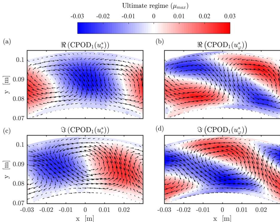
FIGURE 21. **CPOD**<sub>1</sub> for  $Re_S = 6.68 \times 10^4$  and  $\mu = -0.36$  ( $C_4$ ) at the axial height of the vortex center for both velocity components. (a) Real and (c) imaginary part of **CPOD**<sub>1</sub> for the radial velocity component. (b) Real and (d) imaginary part of **CPOD**<sub>1</sub> for the azimuthal velocity component. Black arrows represent the resulting velocity field of **CPOD**<sub>1</sub>.
