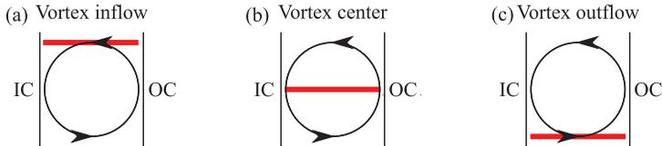
FIGURE 1. Sketch of the ejecting regions bounded by the inner (IC) and outer (OC) cylinders within a Taylor roll: (a) vortex inflow, (b) vortex center, (c) vortex outflow.
