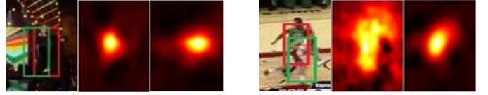
Fig. 2: From left to right: images, response maps without off-line training and response maps with off-line training. Green and red boxes in images indicates tracking results without and with off-line training, respectively.
