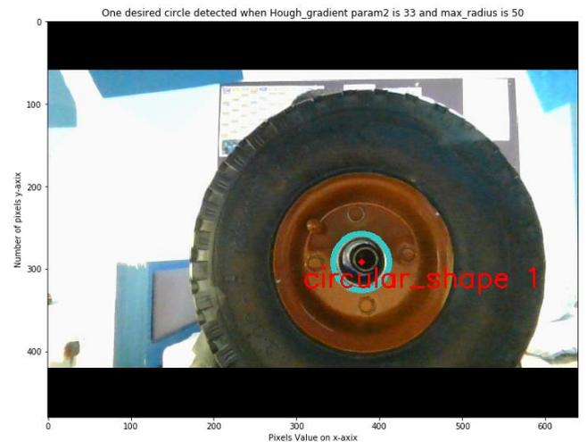
Figure 11: Detected wheel hub with radius of 34 pixels and centre coordinate of [378 292] pixels.
