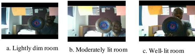
Figure 15: Performance of Camshift Algorithm at about 1m from the Laptop webcam under different lighting condition
