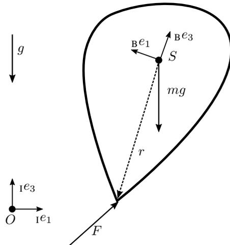
Fig. 2. The figure shows a sketch of the rigid body actuated by the force  $F$ . The body-fixed frame is indicated by the two unit vectors  ${}^B e_1$  and  ${}^B e_3$ . The two unit vectors  ${}^1 e_1$  and  ${}^1 e_3$  belong to the inertial frame of reference. The point  $O$  refers to the origin of the inertial frame of reference, whereas the point  $S$  represents the center of gravity.
