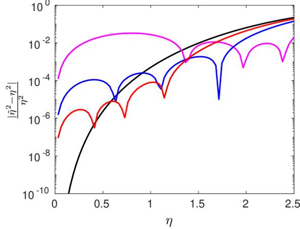
Figure 7: Spectral error for various  $\gamma(\eta)$  for second derivative. Standard eighth order scheme (black),  $\gamma(\eta) = 1$  (magenta),  $\gamma(\eta) = \exp(-\eta/0.1)$  (blue) and  $\gamma(\eta) = \exp(-\eta/0.06)$  (red) for  $\eta \in [0, 2.5]$  and 0 otherwise.
