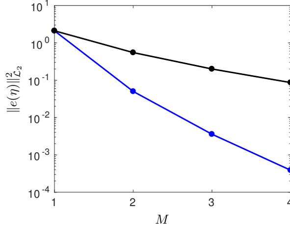
Figure 3: Optimal spectral error for various stencil size  $M$ , approximating second derivative. The blue line corresponds to the second order optimized schemes presented in Fig. 1 and Table 1. The black line corresponds to the standard schemes with stencil size  $M$  and  $2M$  order of accuracy.
