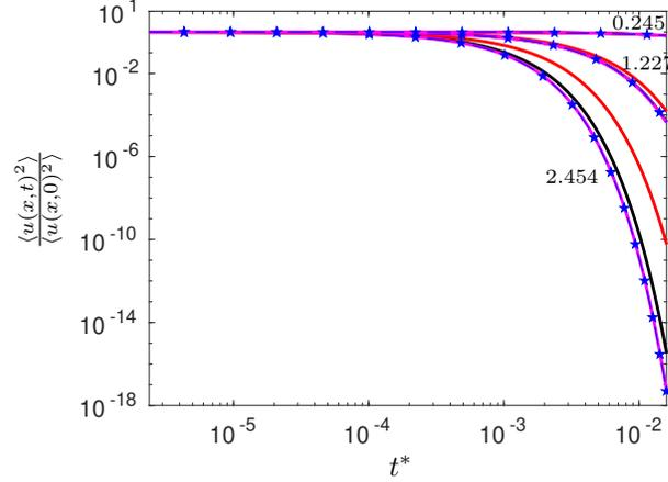
Figure 15: Evolution of space-averaged energy normalized by the initial space-averaged energy with normalized time  $t^* = tc/L$  for three different wave-numbers ( $\eta = 0.245, 1.227, 2.454$ ). Different line styles correspond to different numerical schemes: SFD8 with RK4 in time (black), OFD2 with forward Euler in time (solid magenta), SFD2 with forward Euler in time (red). The blue dashed-star line is the analytical solution.
