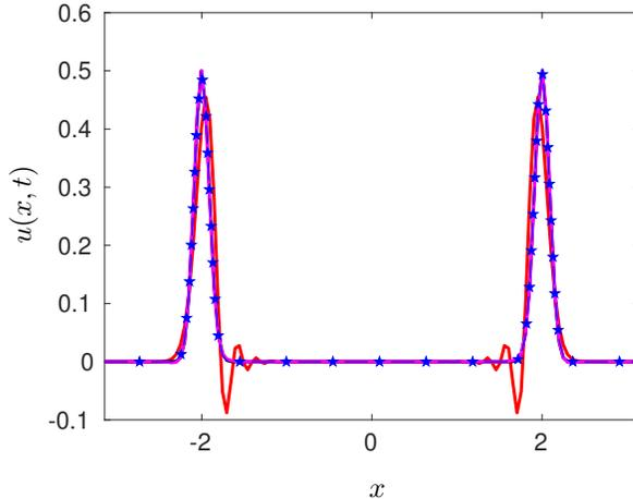
Figure 18: Solution of the wave-equation for  $t = 2$  with a Gaussian initial condition. Different lines correspond to different numerical schemes: SFD8 with RK4 in time (black), OFD2 with RK2 in time (magenta), and SFD2 with RK2 in time (red). The blue dashed-star line is the analytical solution.
