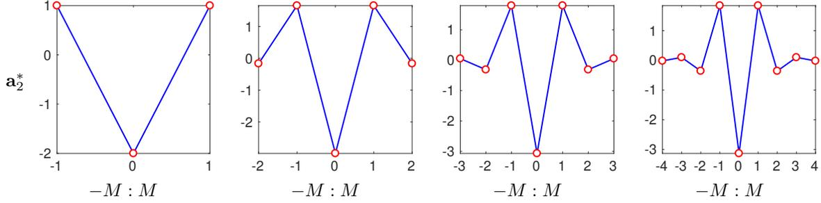
Figure 1: Optimal coefficients for various stencil sizes  $S = 2M + 1$ , for a second derivative with second order accuracy. The coefficients were obtained using  $\gamma(\eta) = 1$ , for  $\eta \in [0, 2.5]$  and  $\gamma(\eta) = 0$  otherwise.
