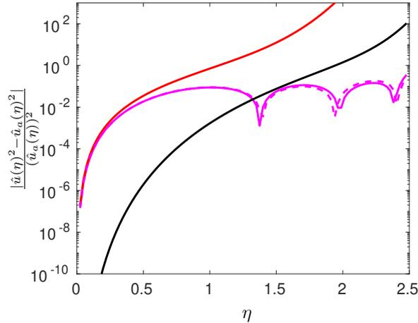
Figure 12: Normalized error in spectral energy for diffusion equation. Solid lines correspond to semi-discrete integration with different numerical schemes: SFD2 (red), SFD8 (black), OFD2 (solid magenta). Dashed magenta line is OFD2 for the fully-discrete system using forward first order in time with  $r_d = 0.0005$ .
