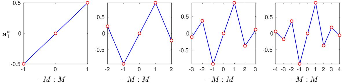
Figure 4: Optimal coefficients for various stencil size  $M$ , approximating first derivative with second order accuracy. The coefficients were obtained using  $\gamma(\eta) = 1$ , for  $\eta \in [0, 2.5]$ ; and  $\gamma(\eta) = 0$  otherwise.
