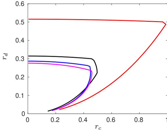
Figure 8: Stability region for the advection-diffusion equation with optimal coefficients  $\mathbf{a}_1^*$  and  $\mathbf{a}_2^*$  for different stencil sizes:  $M = 1$  (red),  $M = 2$  (black),  $M = 3$  (blue),  $M = 4$  (magenta).
