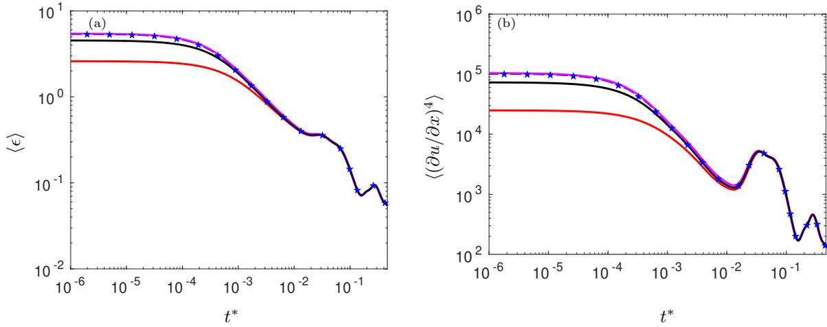
Figure 17: (a) Evolution of space-averaged dissipation (b) Evolution of space-averaged fourth order moment of velocity gradient with normalized time ( $t^* = t/t_0$ ). Different lines correspond to different numerical schemes: SFD8 with RK4 in time (black), OFD2 with forward first-order in time (magenta), and SFD2 with forward first-order in time (red). The blue dashed-star line is the analytical solution.
