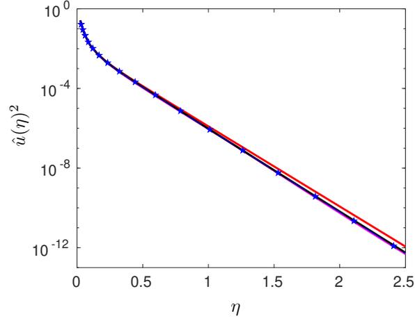
Figure 16: Energy spectrum for the non-linear advection-diffusion equation at  $t^* = t/t_0 \approx 0.464$ . Different lines correspond to different numerical schemes: SFD8 with RK4 in time (black), OFD2 with forward first-order in time (magenta), and SFD2 with forward first-order in time (red). The blue dashed-star line is the analytical solution.
