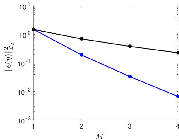
Figure 6: Optimal spectral error for various stencil size  $M,$  approximating first derivative. The blue line corresponds to the second order optimized schemes presented in Fig. 4 and Table 2. The black line corresponds to the standard schemes with stencil size  $M$  and  $2M$  order of accuracy.
