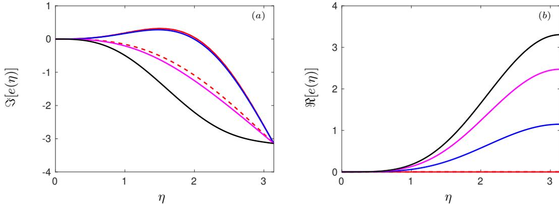
Figure 11: Dispersion error (a) and dissipation error (b) for the first derivative with  $M = 2$  at different values of  $r_c$  and  $r_d$  as marked with the same color in Fig. 10(a). The dashed red line corresponds to standard second order scheme with  $M = 1$  and the dashed magenta line (hidden) corresponds to optimized scheme obtained for  $M = 2$  without stability constraint.
