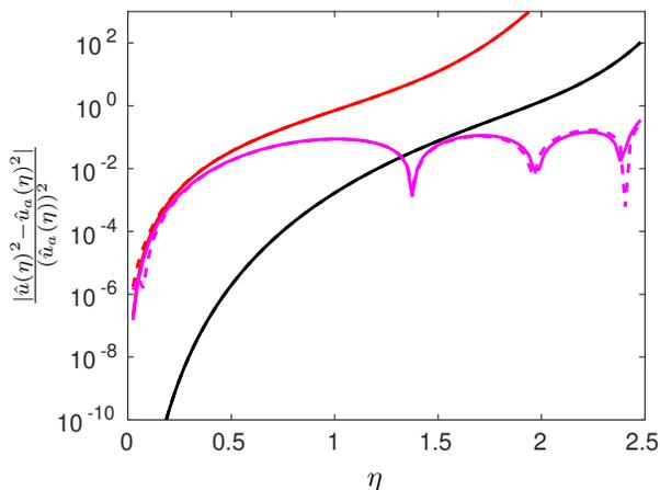
Figure 13: Normalized error in spectral energy for advection-diffusion equation. Different lines correspond to different numerical schemes: standard second order in space (red), standard eighth order in space (black), optimized ( $M-4$ ) second order in space (solid magenta) and optimized ( $M-4$ ) second order in space and forward first order in time (dashed magenta)
