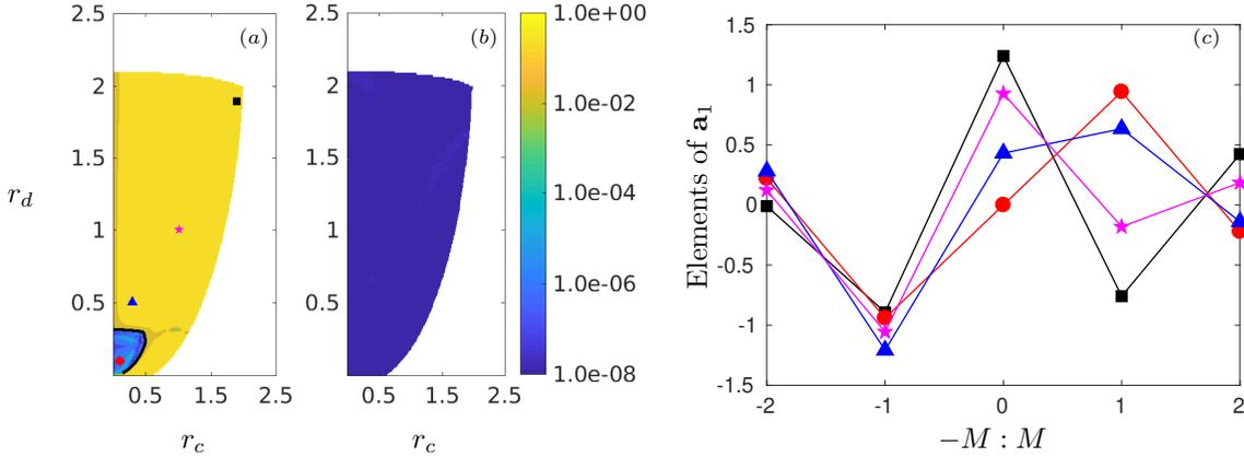
Figure 10: Contours of measure  $A$  for  $M = 2$  for (a) first derivative (b) second derivative. (c) Optimal coefficients for different values of  $r_c$  and  $r_d$  as marked, with the same symbols, in (a).
