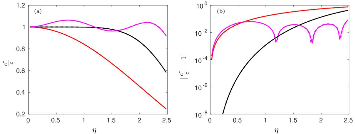
Figure 14: (a) Ratio of numerical to actual speed. (b) Normalized phase error for advection-diffusion equation. Different lines correspond to different numerical schemes: SFD2 (red), SFD8 (black), semi-discrete with OFD2 in space (solid magenta) and OFD2 in space and forward first order in time (dashed magenta).
