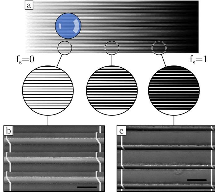
**Figure 7:** Rail geometry used to create gradients of wettability on super-hydrophobic and liquid surfaces. (a) Parallel rails with divergent width along their length. The center-lines of two consecutive rails are separated by 75  $\mu\text{m}$ . The solid surface area evolves from  $f_s = 0$  on the left to  $f_s = 1$  on the right. (b)-(c) SEM images of the divergent rails at two different positions. The scale bars are 75  $\mu\text{m}$ .
