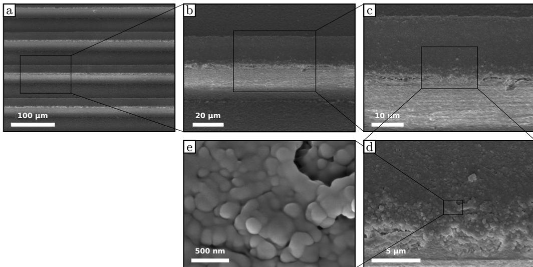
**Figure 5:** SEM images of the micro-structures manufactured by photolithography and coated with a conformal layer of silanized nano-particles. (a) Parallel rails obtained by photolithography. (e) Close-up of the top of a rail highlighting the nano-particles of the porous layer.
