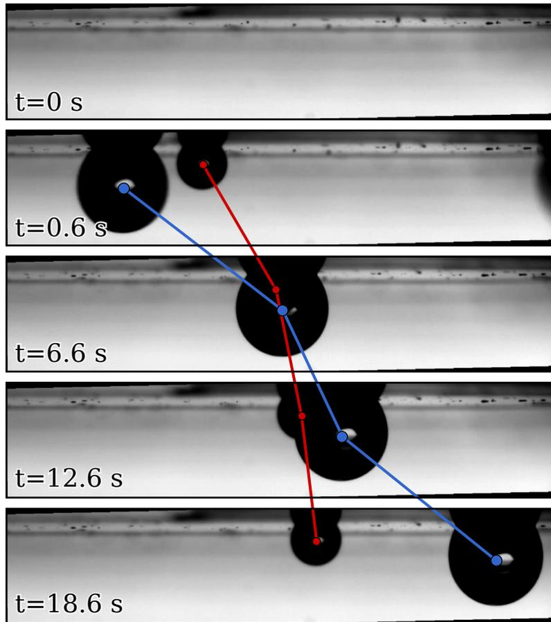
**Figure 11:** Droplets projected on an upside-down shaped liquid surface. Droplets are captured due to the surface high normal adhesion and then driven towards the high wettability region (right here). Droplets of different sizes move at different velocities, in agreement with Fig. 2 from the main manuscript.
