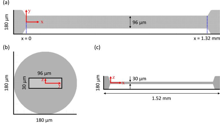
**Figure S10:** Geometry of the computational model (CTRAC-L, larger contraction). (a) is the top view of the geometry, showing the widthwise span of the channel. In (a), the main channel (rectangular) is marked with two blue dotted lines. (b) shows cross-sectional views of the front-end and rear-end of the tapered entry region, the latter of which coincides with the channel entrance ( $x = 0$ ). (c) is the side view of the geometry, showing the depthwise span of the channel.
