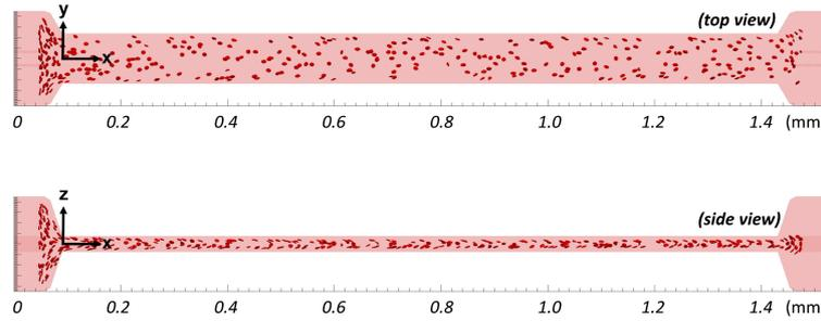
**Figure S11:** A snapshot of the simulation at  $t = 0.37s$ , showing distribution of the 1% RBC suspension in the width and depth directions of the microchannel. Cells arriving at the end of the channel are removed from the system.
