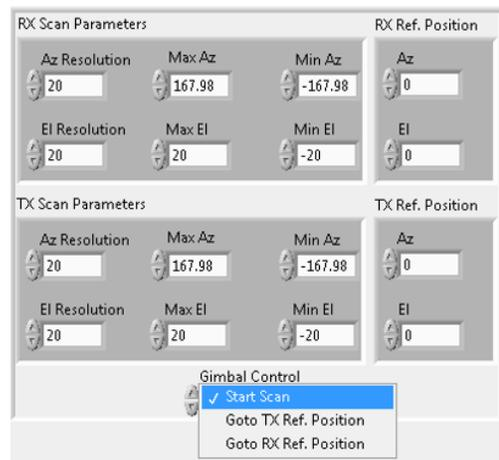
Fig. 4: User interface to control the rotating gimbals.
