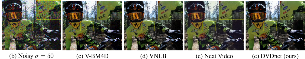
Fig. 3. Comparison of results. Left to right: noisy frame ( PSNR_{seq} = 14.15dB ), output by V-BM4D ( PSNR_{seq} = 24.91dB ), output by VNLB ( PSNR_{seq} = 26.34dB ), output by Neat Video ( PSNR_{seq} = 23.11dB ), output by DVDnet ( PSNR_{seq} = 26.62dB ). Note the clarity of the denoised text, and the lack of low-frequency residual noise and chroma noise for DVDnet. Best viewed in digital format.
