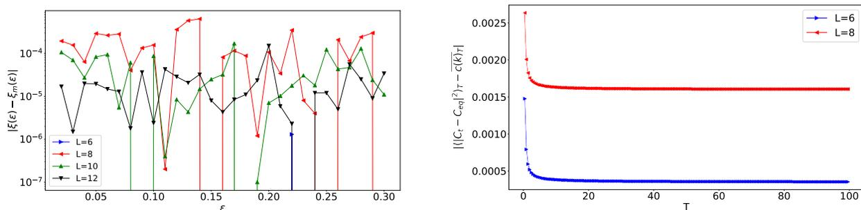
FIG. 3. (left) Forward error plot depicting the accuracy of the Monte Carlo scheme at different values of system size.  $\xi(\epsilon)$  is exactly calculated and  $\xi_m(\epsilon)$  is calculated using the Monte Carlo scheme with 10,000 samples per value of  $\epsilon$ . (right) Forward error plot depicting the accuracy of the integral approximation in calculating the left hand side of equation B23 at various values of time and system size. A step size in time of  $\Delta t = 0.001$  was used.
