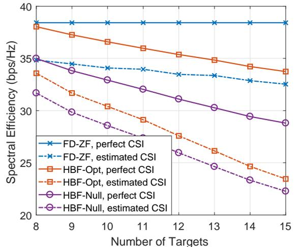
Fig. 9. Tradeoff between the spectral efficiency and the number of targets,  $\text{SNR} = 20\text{dB}$ .
