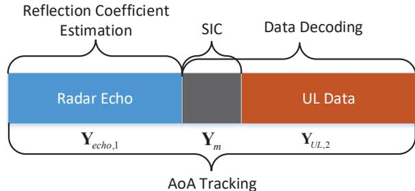
Fig. 3. Overlapped receive signal model.
