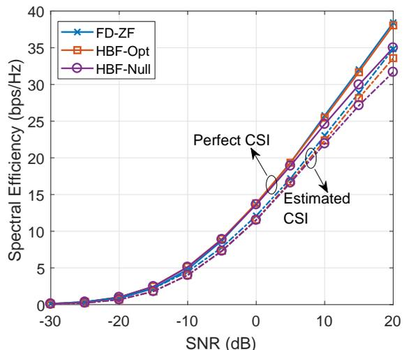
Fig. 7. Spectral efficiency of the DL communication by using (47).
