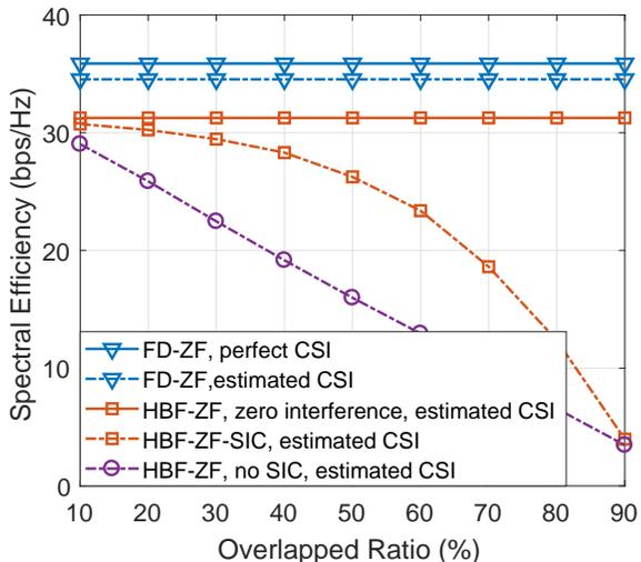
Fig. 11. Tradeoff between the spectral efficiency and the overlapped ratio, SNR = 20dB.
