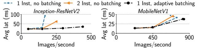
**Figure 3:** Impact of adding model instances versus adaptive batching for two variants on a V100 GPU. Left graph shows average latency and total throughput across 16 threads sending batch-1 requests for Inception-ResNetV2. Right graph is the same for MobileNetV1, 32 threads. Both variants are TensorFlow, batch-8, FP16.
