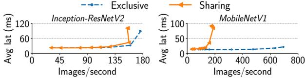
**Figure 5:** Impact of co-locating two models, Inception-ResNetV2 (large) and MobileNetV1 (small), on a V100 GPU. Graphs show average latency and throughput for each model running alone versus sharing. When sharing, same QPS sent to both models. Both variants are TensorRT, batch-1, FP16.
