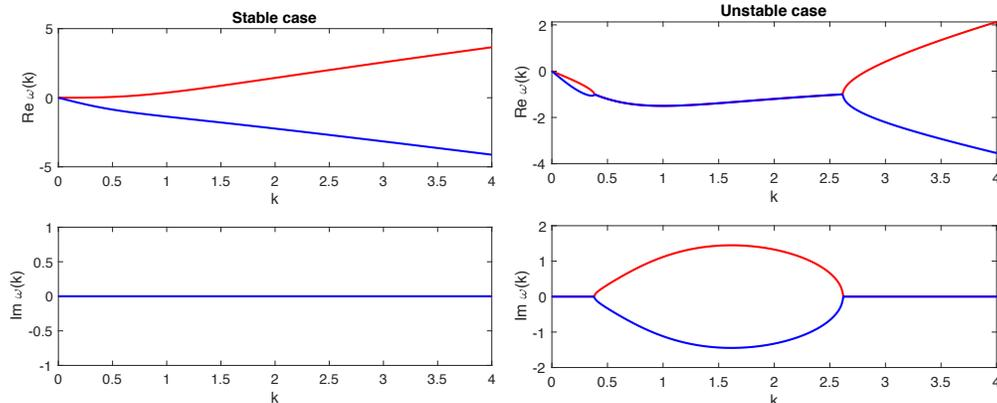
Figure 3.1: Examples of  $\omega(k)$  computed from (3.42), with  $\zeta_0 = 1$ . Left panels:  $U = 1$  (stable case). Right panels:  $\zeta_0 = 0$  (unstable case). Solid red and blue line correspond to the respective choices of the  $+$  and  $-$  sign in (3.42).
