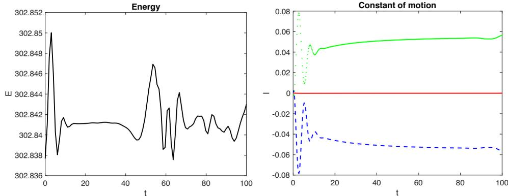
Figure 3.3: Computed value of the conserved quantities for simulation shown on Figure 3.2. Left panel: energy  $E$  as defined in (3.33). Right panel: quantity defined by (3.36) Dashed blue line:  $\int B_t ds$ . Dotted green line:  $\int B_{ss} B_{ts} ds$ . Solid red line: the conserved quantity  $I = \int B_t + B_{ss} B_{ts} ds$ .
