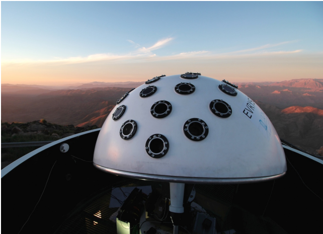
Figure 1. The Evryscope, a two-dozen-camera array mounted into a 6 ft-diameter hemisphere, deployed at the CTIO observatory.
