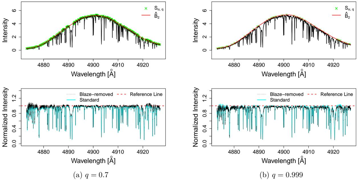
**Figure 7.** Comparison of the results of the AFS algorithm using extreme values for the  $q$  parameter. (a) Small  $q$ : 0.7. (b) Large  $q$ : 0.999. The cyan spectrum shows the results from the standard value of  $q = 0.95$ .
