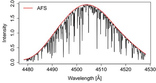
(a) A blue order of NSO simulated spectrum, S/N 300, temperature 5778 K, metallicity 0 dex:  $q = 0.99$ ,  $m_0 = 0.3$
