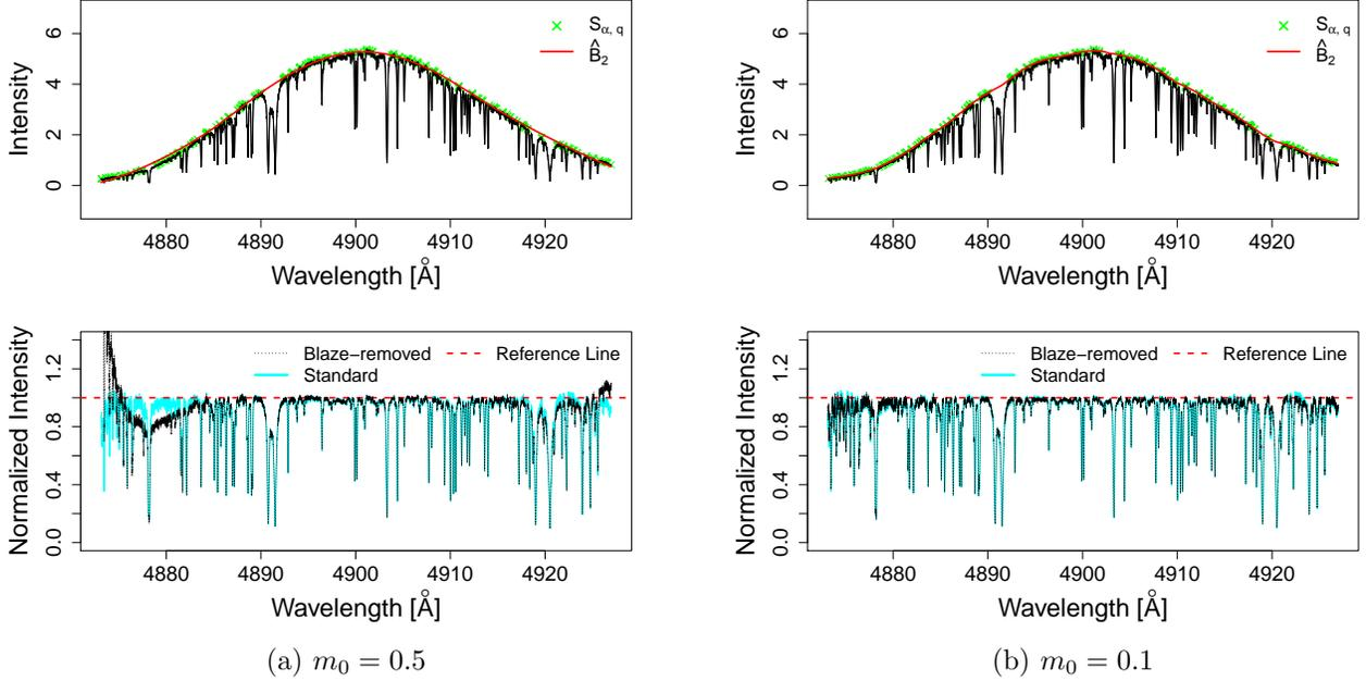
**Figure 8.** Comparison of the results of the AFS algorithm using extreme values for the  $m_0$  parameter. (a) Large  $m_0$ : 0.5. (b) Small  $m_0$ : 0.1. The cyan spectrum shows the results from the standard value of  $m_0 = 0.25$ .
