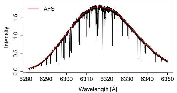
(f) A red order of NSO simulated spectrum, S/N 50, temperature 5778 K, metallicity 0 dex:  $q = 0.5$ ,  $m_0 = 0.25$
