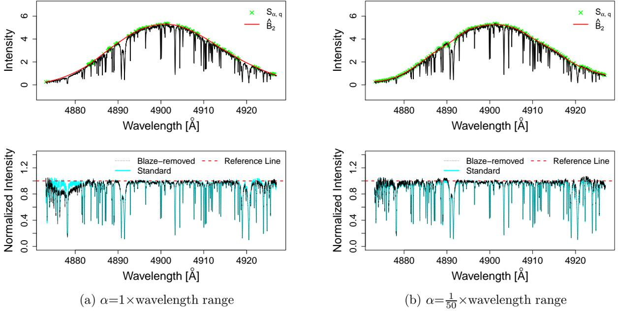
**Figure 6.** Comparison of the results of the AFS algorithm using extreme values for the  $\alpha$  parameter. (a) Large  $\alpha$ :  $1 \times \text{wavelength range}$ . (b) Small  $\alpha$ :  $\frac{1}{50} \times \text{wavelength range}$ . The cyan spectrum shows the results from the standard value of  $\alpha = \frac{1}{6} \times \text{wavelength range}$ .
