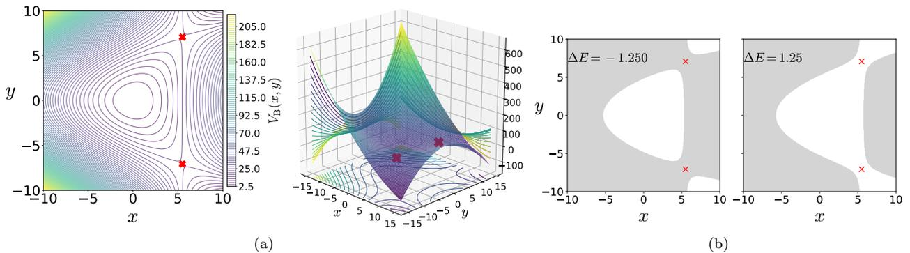
FIG. 1. (a) Potential energy function underlying the coupled harmonic Hamiltonian (1) as isopotential contour and surface. The index-1 saddles are shown as red crosses in both the plots. (b) Hill's region for energy below and above the energy of the index-1 saddle. Parameters used are  $\omega_x = 1.0, \omega_y = 1.1, \delta = -0.11$ .
