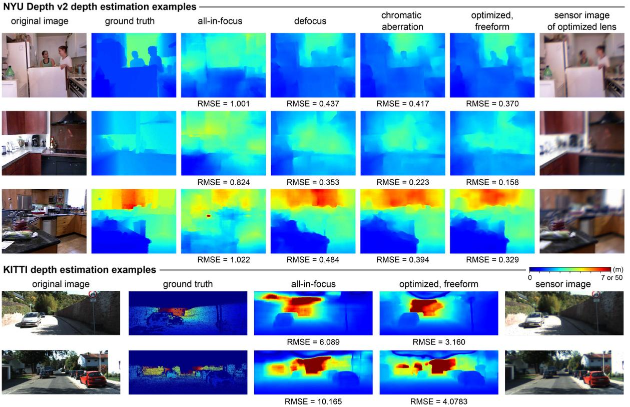
Figure 4. **Depth estimation.** (Top) Examples with RMSE (m) from the NYU Depth v2 dataset with all-in-focus, defocus, chromatic aberration, and optimized models. The simulated sensor image from the optimized system is also shown. (Bottom) Examples with RMSE (m) from the KITTI dataset (cropped to fit) with all-in-focus and optimized models; the sensor image from the optimized model is also shown. All depth maps use the same colormap, but the maximum value is 7 m for NYU Depth and 50 m for KITTI.
