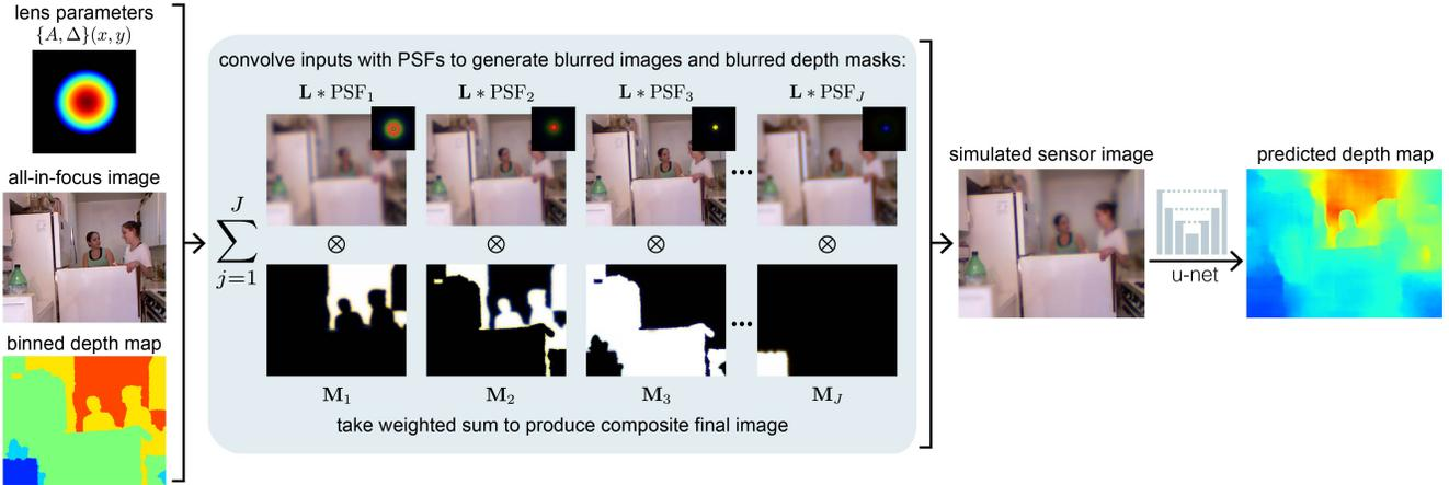
Figure 3. **Depth-dependent image formation.** Given a set of lens parameters, an all-in-focus image, and its binned depth map, the image formation model generates the appropriate PSFs and applies depth-dependent convolution to simulate the corresponding sensor image, which is then passed into a U-Net for depth estimation.
