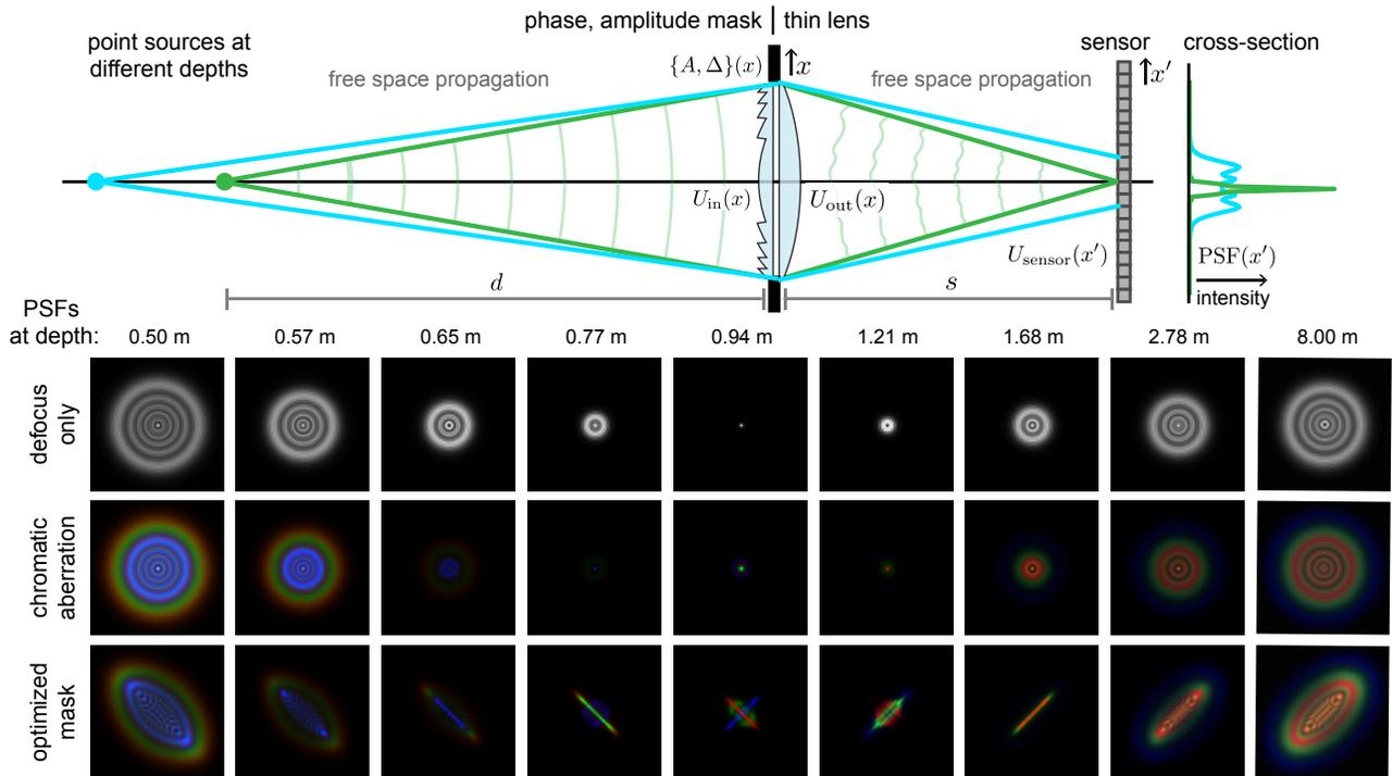
Figure 2. **PSF simulation model.** (Top) Optical propagation model of point sources through a phase mask placed in front of a thin lens. PSFs are simulated by calculating intensity of the electric field at the sensor plane. (Bottom) Sample PSFs from thin lens defocus only, with chromatic aberrations, and using an optimized mask initialized with astigmatism.
