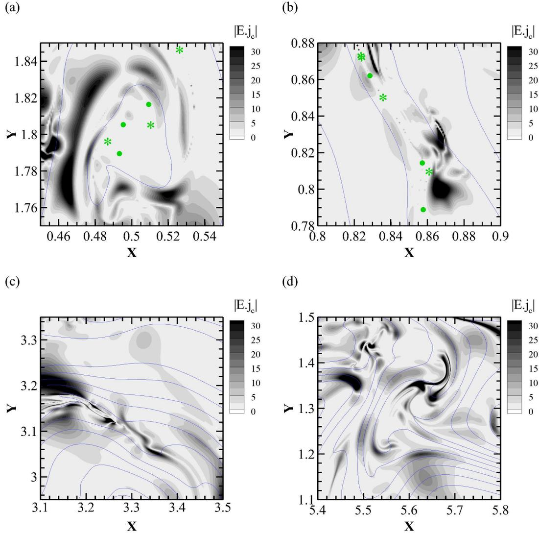
FIG. 6. Contour maps of the curvature drift acceleration term  $|\mathbf{E} \cdot \mathbf{j}_c|$ . (a) and (b): regions with magnetic island cores marked as green circles and magnetic reconnection sites marked as green stars. (c) and (d): regions that do not contain topologically special points. The blue contour lines show the magnetic field lines.
