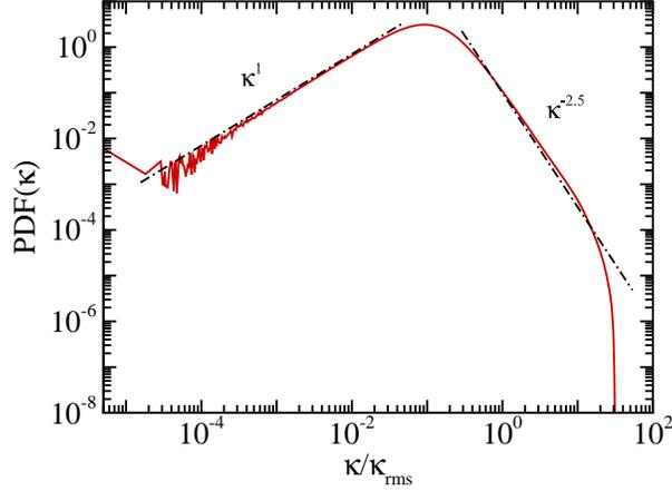
FIG. 7. 3D MHD simulation: PDF of the magnetic field curvature  $\kappa$  normalized to the root mean square value  $\kappa_{\text{rms}}$ . The PDF has a  $\kappa^1$  low-curvature regime and a  $\kappa^{-2.5}$  high-curvature tail.
