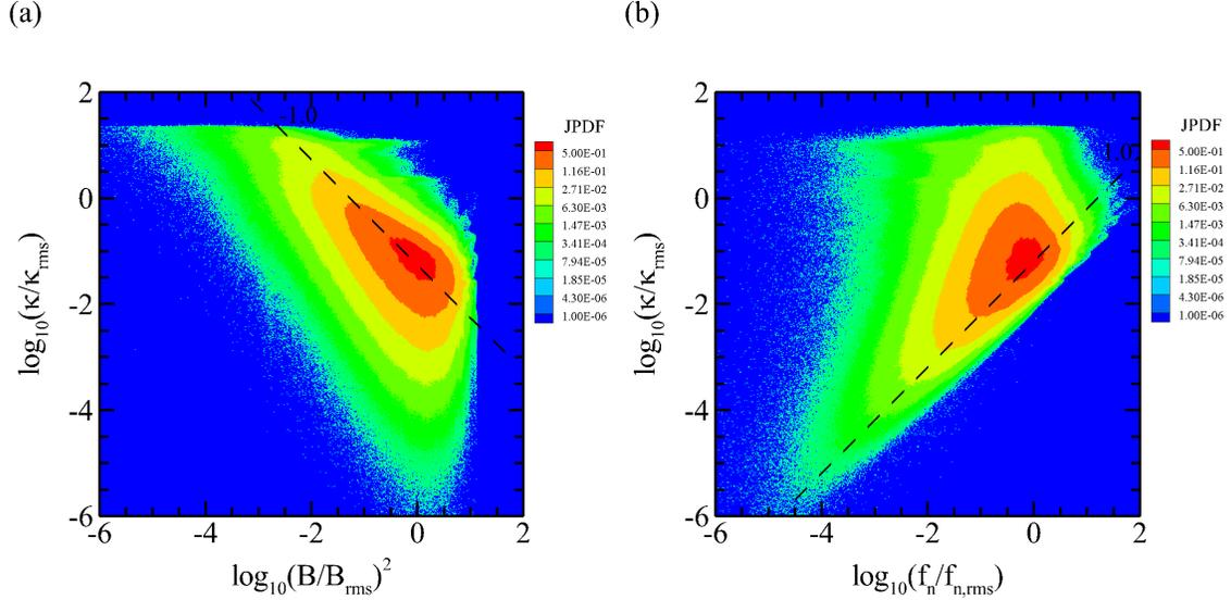
FIG. 2. Joint PDFs of the curvature  $\kappa$  and (a) the square of magnetic magnitude  $B^2$  and (b) the force magnitude  $f_n$  acting normal to field lines. All quantities are normalized to their respective root mean square values. There are apparent associations between high curvature and low magnetic field and between low curvature and low normal force.
