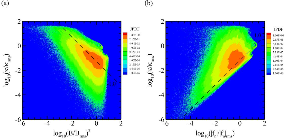
FIG. 10. PIC simulation: Joint PDFs of the curvature  $\kappa$  and (a) the square of magnetic magnitude  $B^2$  and (b) the force magnitude  $f_n$  acting normal to field lines.
