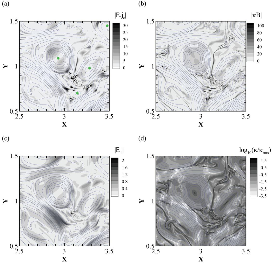
FIG. 4. Contour maps of (a) the curvature drift acceleration term  $|\mathbf{E} \cdot \mathbf{j}_c|$ , (b) the curvature-related component  $|\kappa B|$ , (c) the perpendicular electric field  $|E_\perp|$ , and (d) the logarithm of the curvature  $\kappa$  in a subregion of the whole domain with the blue contour lines showing the magnetic field lines.
