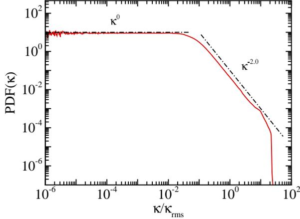
FIG. 1. PDF of the magnetic field curvature  $\kappa$  normalized to the root mean square value  $\kappa_{\text{rms}}$ . The PDF has a  $\kappa^0$  low-curvature regime and a  $\kappa^{-2}$  high-curvature tail.
