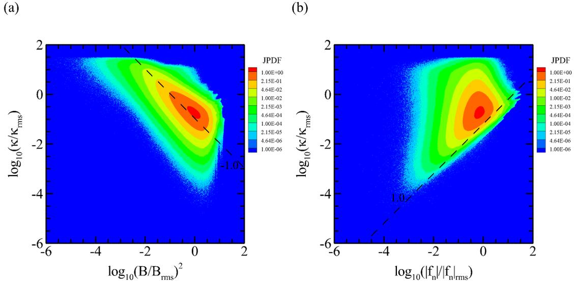
FIG. 8. 3D MHD simulation: Joint PDFs of the curvature  $\kappa$  and (a) the square of magnetic magnitude  $B^2$  and (b) the force magnitude  $f_n$  acting normal to field lines. All quantities are normalized to their respective root mean square values. There are apparent associations between high curvature and low magnetic field and between low curvature and low normal force.
