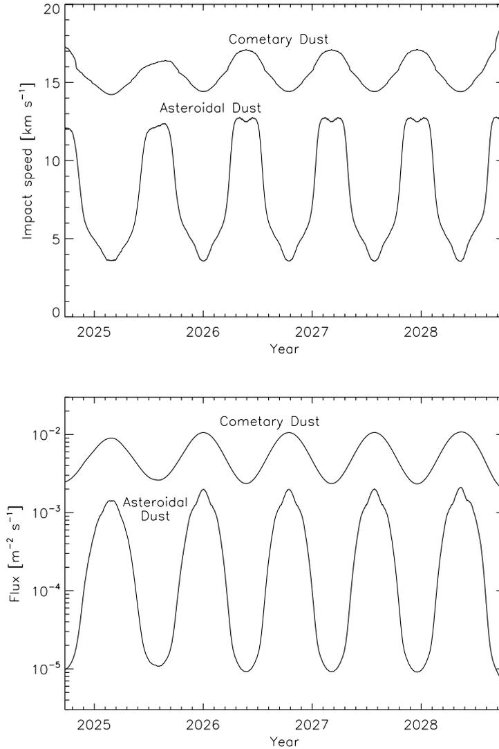
Figure 3: Average particle impact speed (*top panel*) and flux (*bottom panel*) of asteroidal dust (population 2) and cometary dust (population 4) on to DESTINY<sup>+</sup> in the spacecraft reference frame, for a flat plate sensor whose normal vector points parallel to the spacecraft velocity vector (continuous apex pointing).
