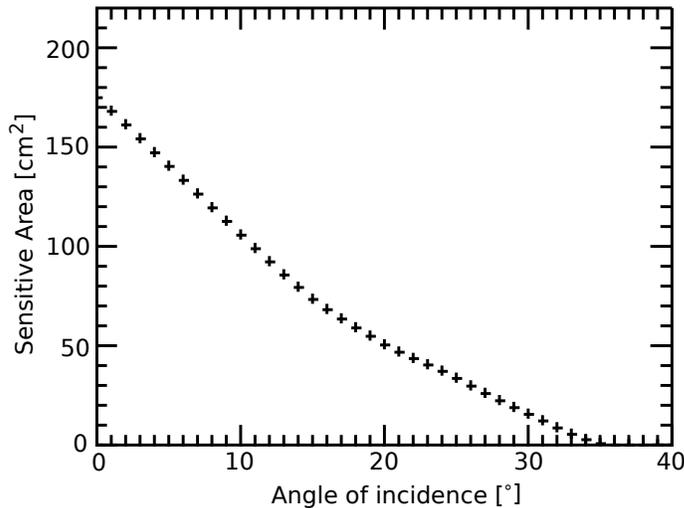
Figure 5: Field-of-view for DDA used for IMEM and IMEX simulations. The sensitive area refers to a single DDA sensor head.
