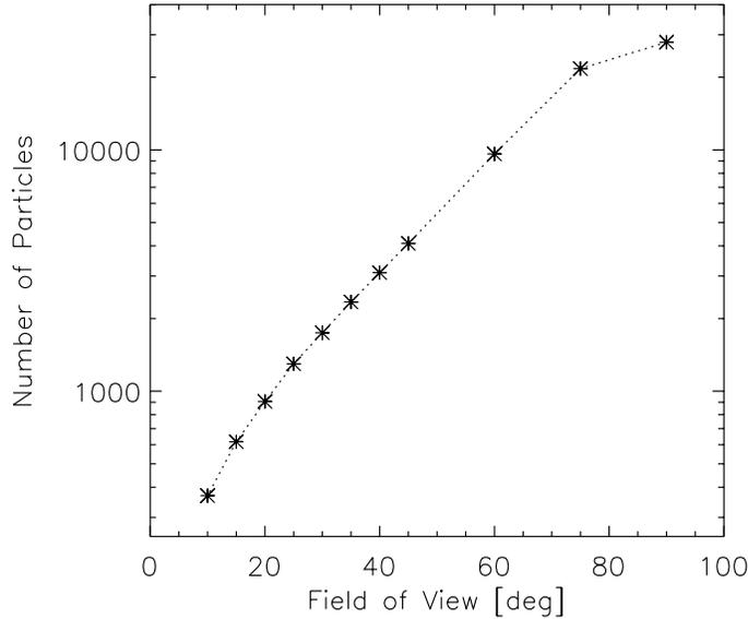
Figure 6: Fluence of interplanetary dust particles for a flat plate sensor with  $0.035\text{ m}^2$  sensor area and varying sensor FOVs from IMEM simulations. The DDA field-of-view corresponds to an angle of  $17^\circ$  in this diagram.
