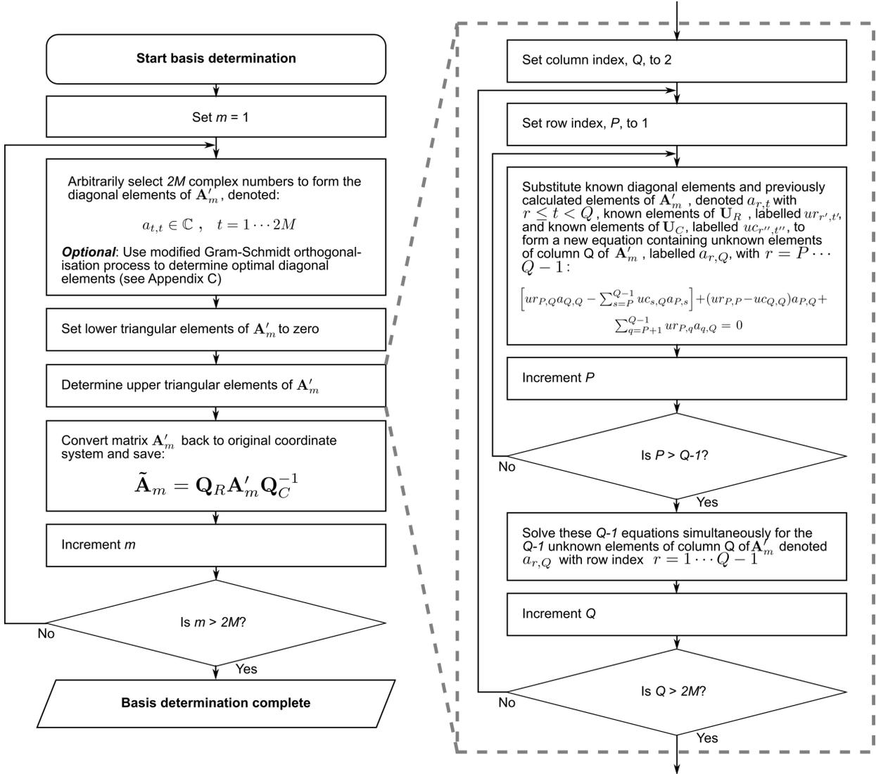
FIG. 14. Flowchart detailing the process of finding a basis for the matrix  $\mathbf{A}$  using the zeroth-order solution method.
