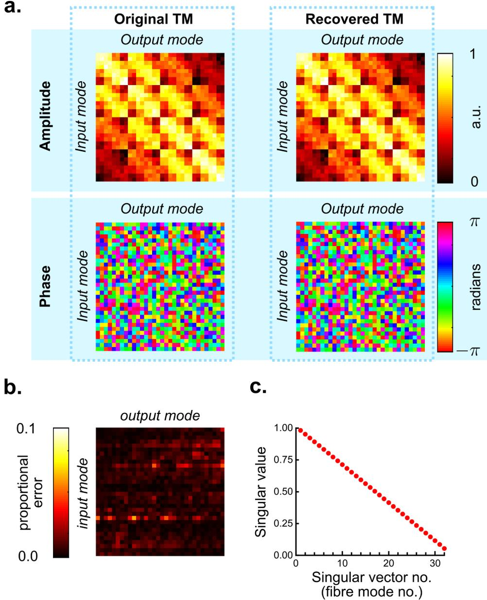
FIG. 5. **Recovery of a simulated TM using the first-order recovery algorithm:** a) The original simulated TM is compared with the recovered TM (noise level  $\sigma_n = 10^{-3}$ ) demonstrating successful recovery. b) Proportional element-wise error in TM reconstruction (maximum  $< 0.05$ ) after 300 iterations of first-order model. c) Singular values of TM demonstrating non-unity.
