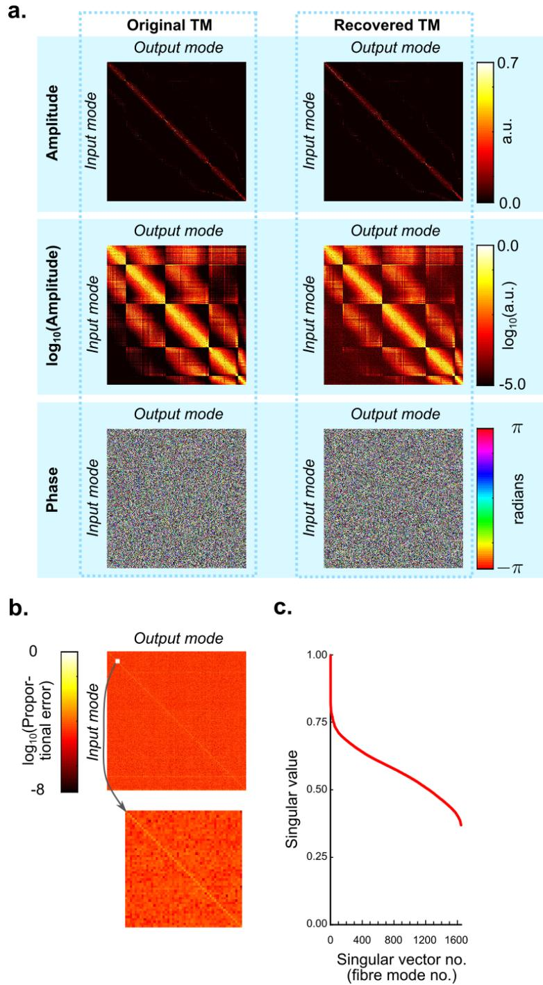
FIG. 7. **First-order recovery of an experimentally-measured MCF TM.** a) Original TM using data from [3] and the first-order recovered TM, showing high visual similarity indicating successful recovery. b) Proportional element-wise error in TM reconstruction (maximum  $< 10^{-3}$ ). c) Singular values of TM demonstrating non-unitarity.
