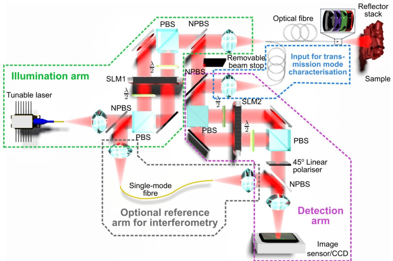
FIG. 10. **Conceptual experimental set-up for fibre TM characterisation in reflection mode configuration using distal reflector stack.** SLM: spatial light modulator, PBS: polarising beam splitter, NPBS: non-polarising beam splitter,  $\lambda/2$ : half waveplate.
