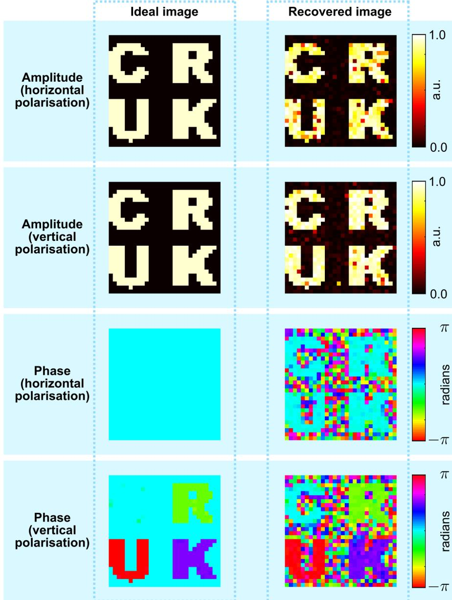
FIG. 8. **Successful reconstruction of an amplitude, phase and polarisation image of a target at the distal facet using a TM recovered using the first-order model.** The recovered image noise is largely driven by illumination correction (see Section IID).
