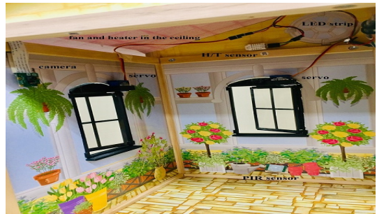
Fig. 7: Picture of one room including its actuators and sensors
