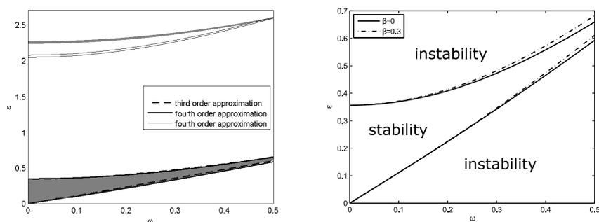
**Fig. 1.** Comparison of approximate stability boundaries of the third (dashed lines) and fourth (solid lines) orders with exact stability domains (gray areas) on the left. Damping stabilization and destabilization of the inverted vertical pendulum position on the right.
