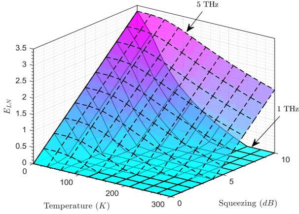
Fig. 2. The logarithmic negativity  $E_{LN}$  of a two-mode squeezed thermal state against system temperature and squeezing for frequencies of 1THz and 5THz. It should be noted that no losses are assumed here.
