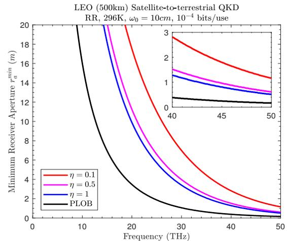
Fig. 6. Minimum receiver aperture radius versus QKD frequencies. Multiple detection efficiencies are considered. The PLOB bound with  $\eta = 1$  is considered for comparison. Here we set  $\omega_0 = 10cm$ .
