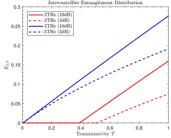
Fig. 3. The output entanglement  $E_{LN}(\rho_{out})$  for inter-satellite entanglement distribution against the channel transmissivity  $T$ . The solid lines refer to 10dB initial squeezing, and the dashed lines refer to 3dB initial squeezing. Two THz frequencies, namely 2THz and 5THz, are considered.
