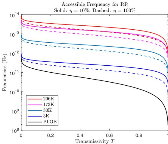
Fig. 5. The accessible frequency against transmissivity for the RR-based inter-satellite QKD protocol at different temperatures. The solid lines refer to the realistic detection efficiency ( $\eta = 10\%$ ), and the dashed lines refer to the ideal detection efficiency ( $\eta = 100\%$ ). The lower bound on the accessible frequency is calculated at 30K for comparison.
