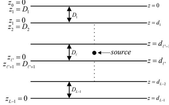
FIG. 3. Sketch of the layer structure for general multi-layer media.
