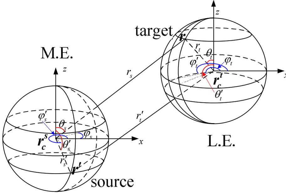
FIG. 1. Spherical coordinates used in multipole and local expansions.
