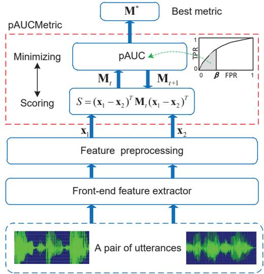
Fig. 3: Diagram of the pAUCMetric based speaker verification system.
