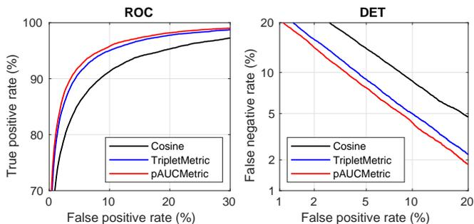
Fig. 7: ROC and DET curves of the comparison methods with the x-vector front-end of the 8 kHz system on the Cantonese data of SRE16.
