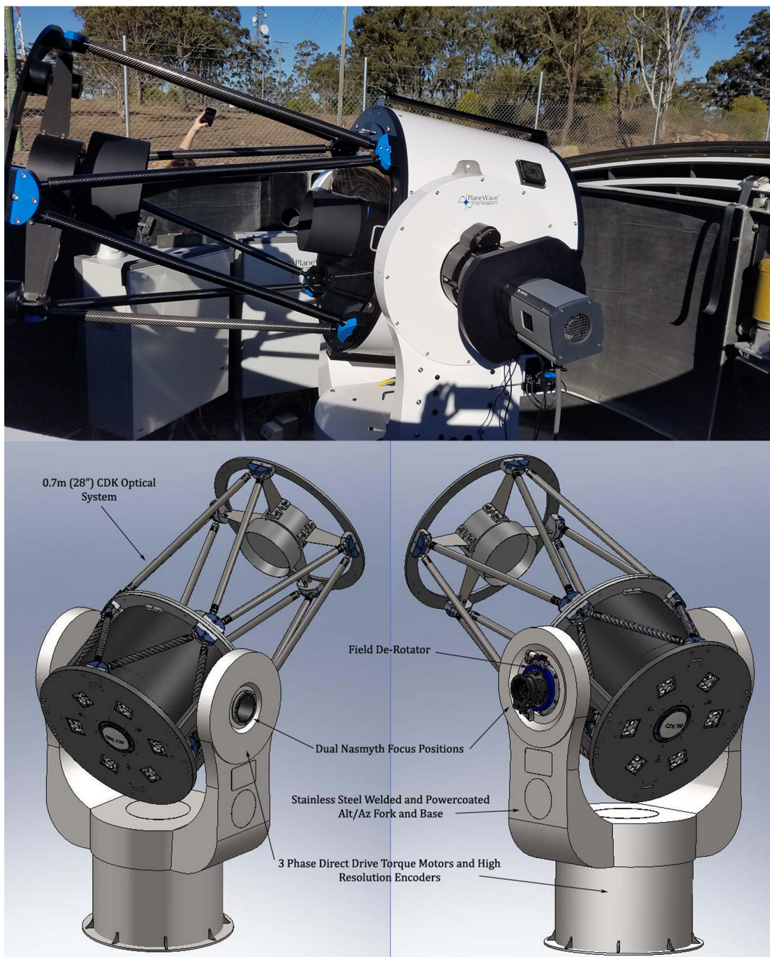
Figure 2. Top: MINERVA-Australis PlaneWave CDK-700 telescope inside an AstroHaven Enterprises Dome. Bottom: schematic of the PlaneWave CDK-700 telescope obtained from the PlaneWave website.
