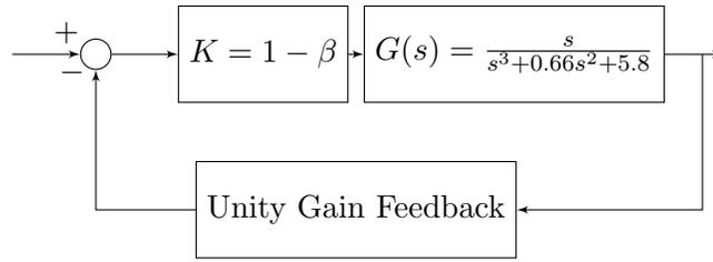
FIG. 7. Block diagram of control loop for root locus analysis of characteristic polynomial of matrix  $A_1$ . The trajectory of the roots of the loop transfer function are analyzed in complex plane as the gain parameter  $K$  is varied from 0 to  $+\infty$ .
