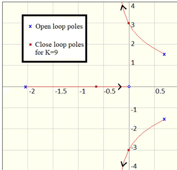
FIG. 8. Root locus for controller shown in Figure 7. The roots lie in the left half of the complex plane for values of gain  $K \geq 9$ .
