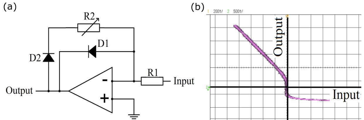
FIG. 2. (a) Circuit diagram for the “f-block” in Figure 1, that implements the equation for  $f(x)$  as in equation (9). (b) Experimentally measured transfer function of the non-linear f-block, verified by applying sinusoidal signal to the f-block circuit and observing output vs input graph on oscilloscope (configured to display in XY mode).
