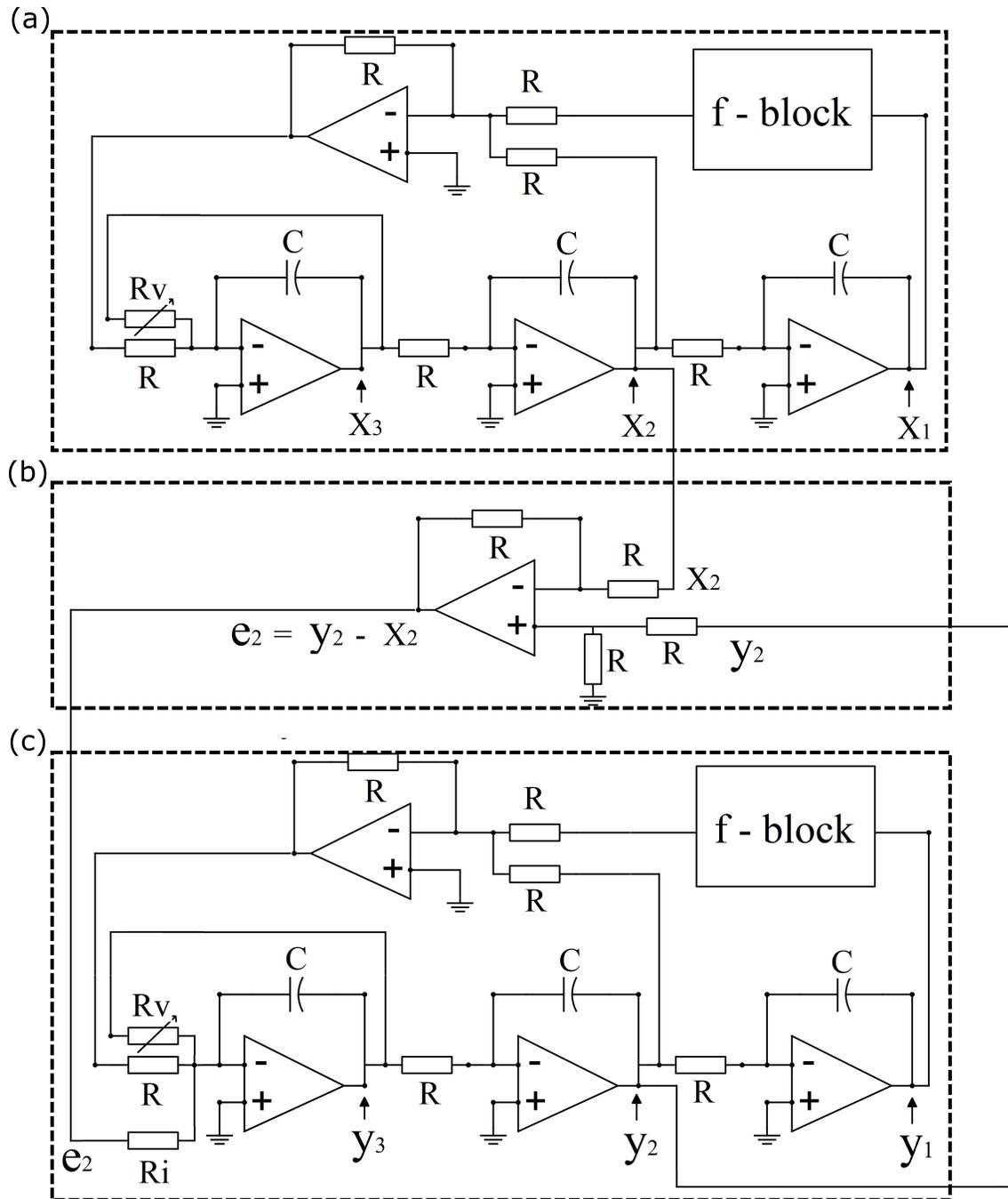
FIG. 9. Circuit diagram showing the (a) master chaotic circuit, (b) linear controller circuit, and (c) slave chaotic circuit with feedback controller:  $u(t) = -\frac{R}{R_i}e_2(t)$
