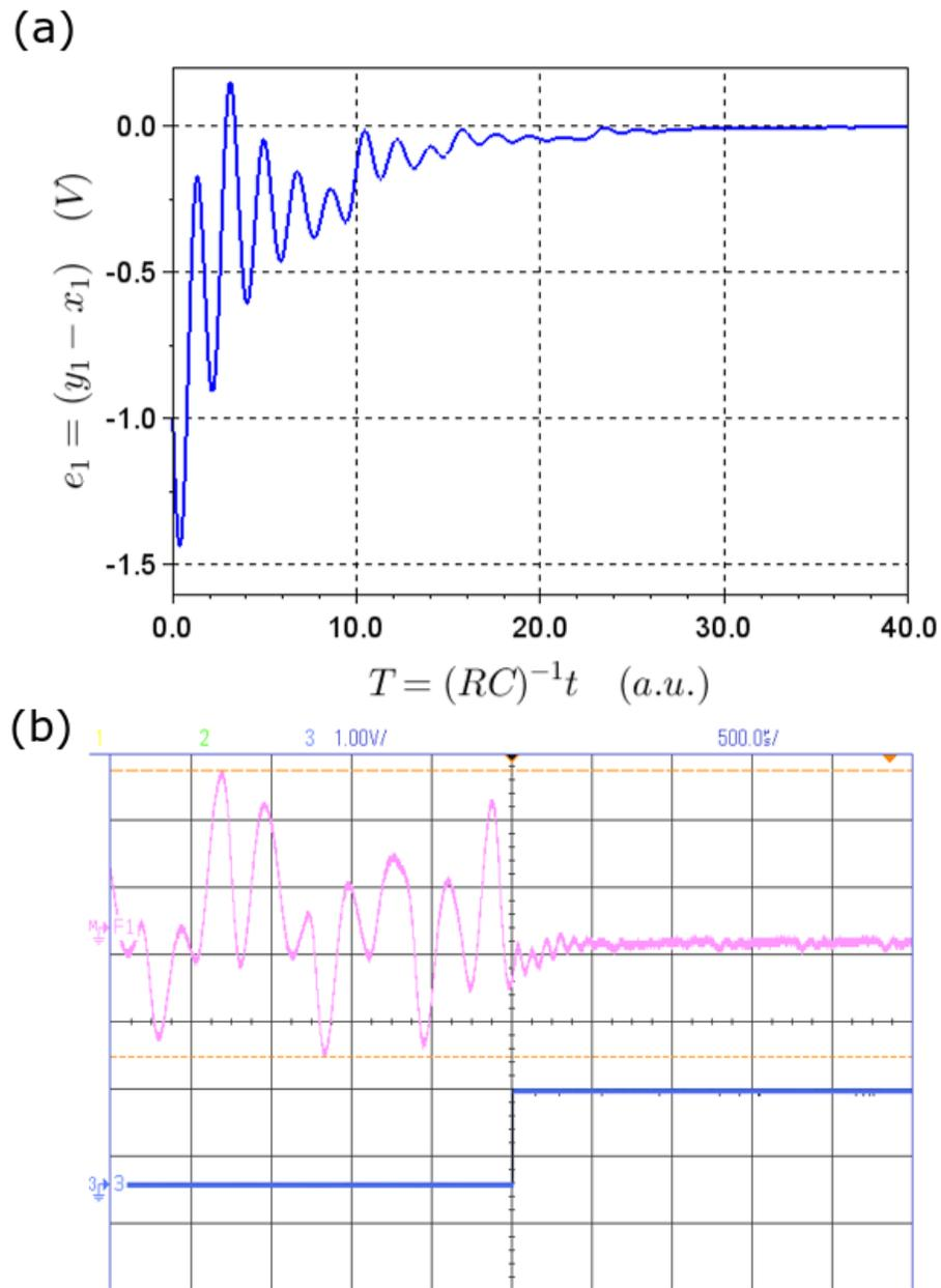
FIG. 10. Response time of controller: (a) Numerical simulation (in Scilab) shows the error state  $e_1$  converging to zero after connecting the control signal  $u(t) = -10e_2(t)$  at time  $T = 0$ . (b) Experimental result observed on an oscilloscope, wherein the error state  $e_1$  converges to zero (upper trace) when the control signal is turned on using an electrical switch gated by the voltage step signal shown in the bottom trace.
