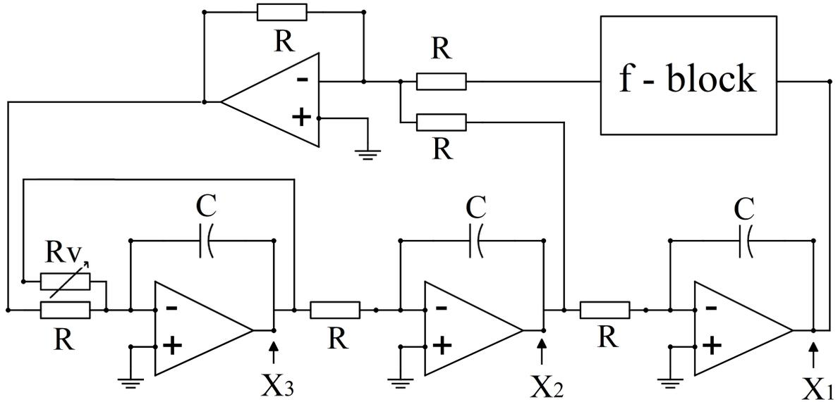
FIG. 1. Circuit diagram of the chaotic signal generator (oscillator), based on an architecture proposed by Kiers et al.<sup>7</sup>. The “f-block” is a non-linear circuit shown in Figure 2.
