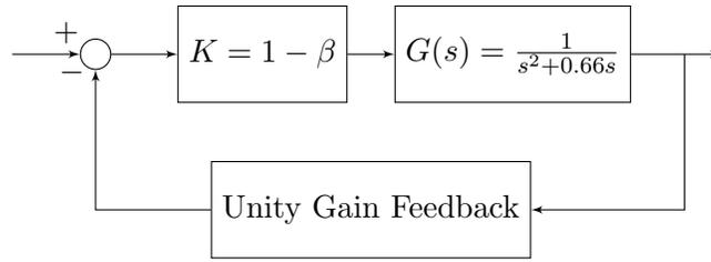
FIG. 5. Block diagram of control loop for root locus analysis of characteristic polynomial of matrix  $A_0$ . The trajectory of the roots of the loop transfer function are analyzed in complex plane as the gain parameter  $K$  is varied from 0 to  $+\infty$ .
