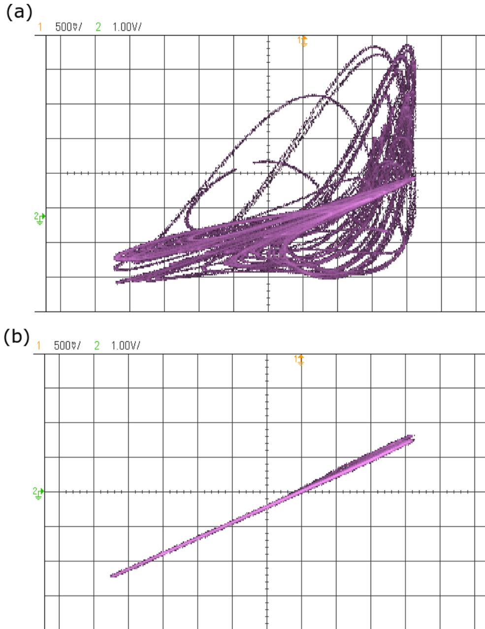
FIG. 11. Signals  $x_1$  (master oscillator, Y-axis) and  $y_1$  (slave oscillator, X-axis) observed on an oscilloscope configured to display in  $XY$  mode. (a) In the unsynchronized state, the two signals are not correlated to each other. (b) When the two oscillators are synchronized, the two signals track each other and are equal in magnitude.
