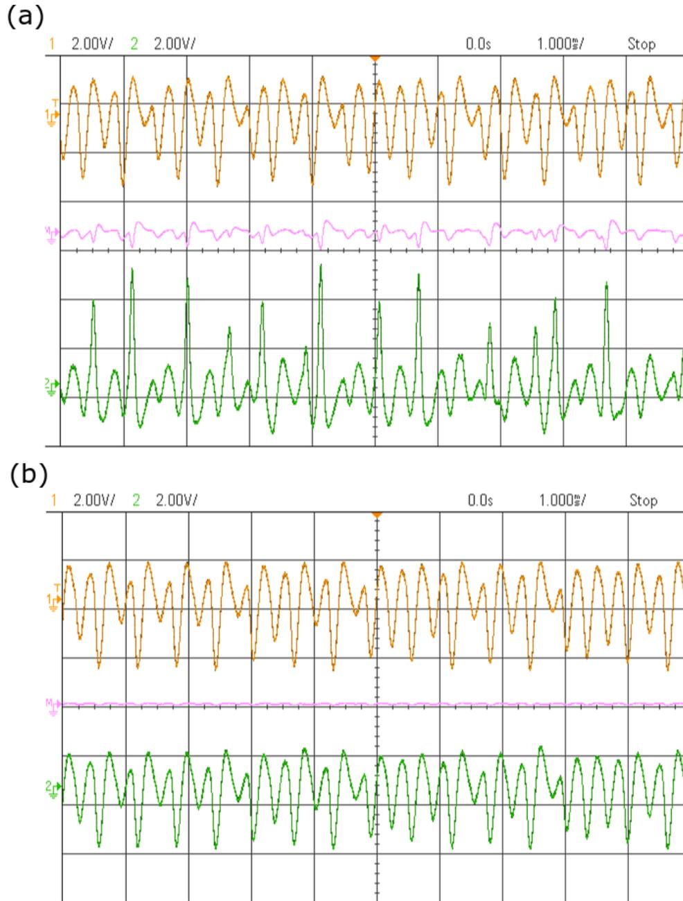
FIG. 12. Signals  $x_1$  (master oscillator, upper trace),  $y_1$  (slave oscillator, bottom trace) observed on an oscilloscope configured to display in time domain. The difference between the two signals is computed and displayed on the oscilloscope (middle trace). (a) When the two oscillators are not synchronized, the difference is non-zero. (b) The difference between  $x_1$  and  $y_1$  is very small, and the two traces look identical when the oscillators are synchronized.
