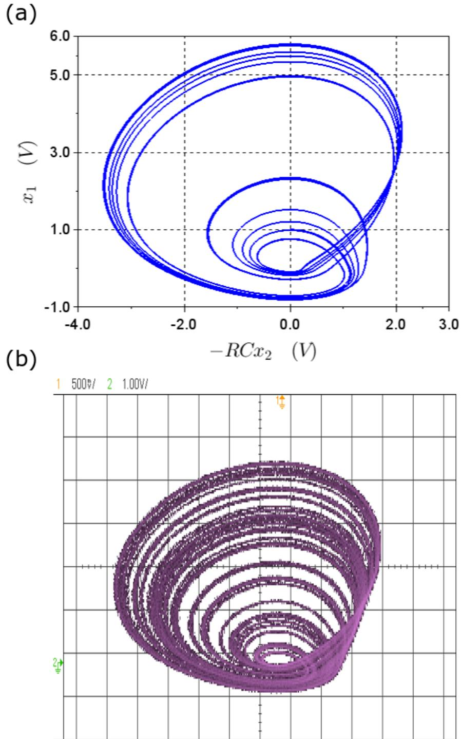
FIG. 4. (a) Simulated phase portrait of the oscillator described in equation (18), obtained using numerical simulation in Scilab. (b) Experimentally measured phase portrait of the oscillator on an oscilloscope configured to display in  $XY$  mode. The Y-axis displays signal at the node  $x_1$  and X-axis displays signal at node  $x_2$ .
