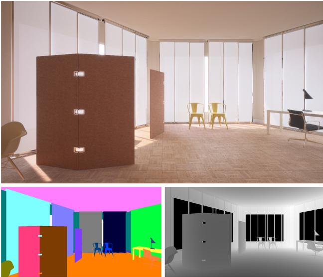
Fig. 6. RGB, instance segmentation masks, and depth map generated with UnrealROX for a synthetic scene rendered in Unreal Engine 4 (UE4).
