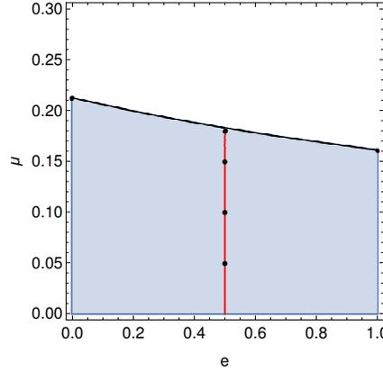
**Figure 4.** The shaded region depicts the bound orbit region defined by Eq. (13c) in the  $(e, \mu)$  plane for  $a = 0.5$  and  $Q = 5$ . The black curve represents the homoclinic orbits where the end points depict  $e = 0$  and  $e = 1$  homoclinic orbits corresponding to the ISSO and MBSO respectively. The red curve represents  $e = 0.5$  and we study orbits with different  $\mu$  values as depicted by the dots on this curve.
