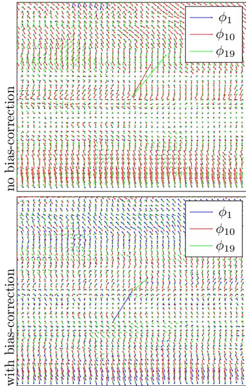
Figure 5: Displacement components of  $\phi_1$ ,  $\phi_{10}$  and  $\phi_{19}$  corresponding to the reconstruction results from Fig. 2. The large arrows in the center show the global translation component of the displacements, the small vectors visualize the local displacement after subtracting the global translation component. All vectors are scaled by a factor of 10 for the purpose of visualization.
