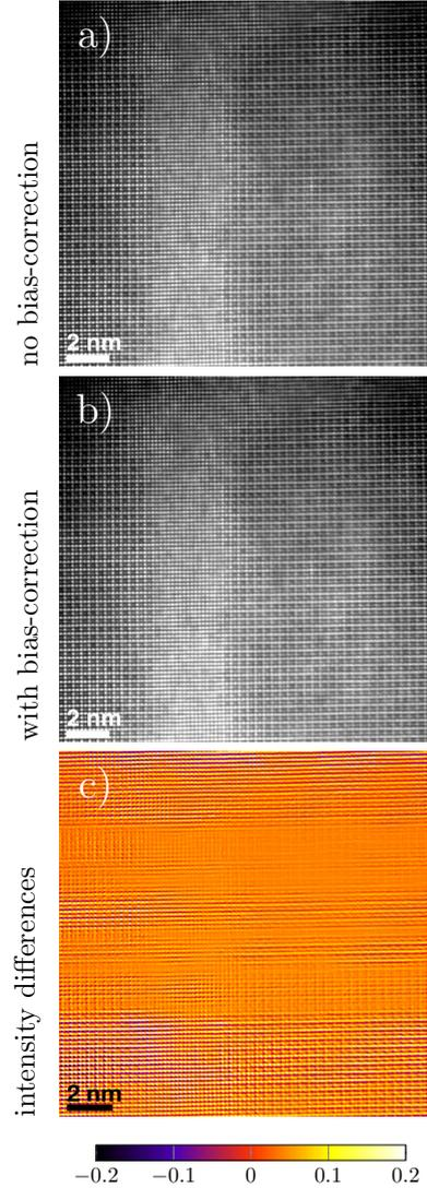
Figure 2: Average of raw images from a serial acquisition scheme of 20 individual images aligned by non-rigid registration without a) bias-correction and b) with bias-correction. The normalized difference image of a) and b) is given in c).
