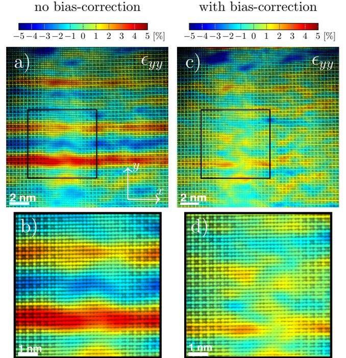
Figure 4: The left and right column display the  $\epsilon_{yy}$  strain component of the non-rigid registration approach without and with bias-correction, respectively. a) and c) illustrate the complete strain maps with the local coordinate system and b) and d) show magnified subregions as indicated by the black rectangles in a) and c).
