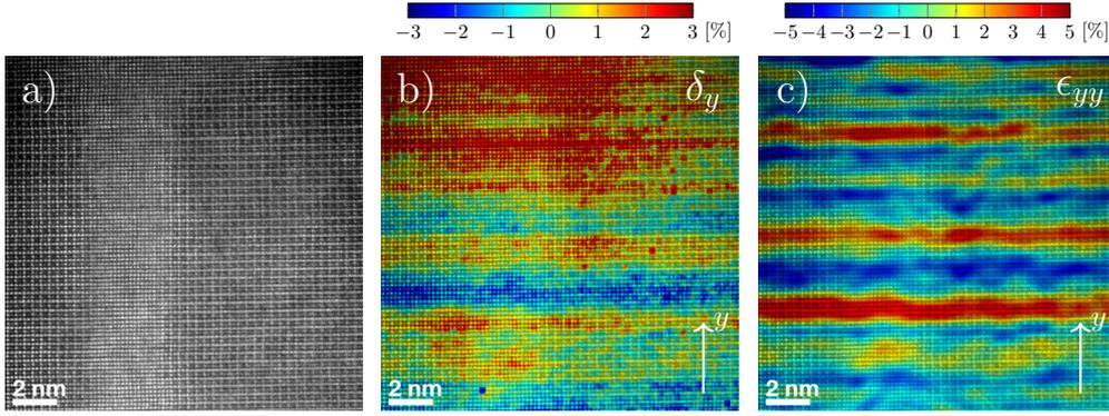
Figure 6: a) HAADF-STEM image of the first frame of the image series. b) Corresponding  $y$ -component of peak displacements  $\delta_y$ . c) Resulting  $\epsilon_{yy}$  strain map determined from the peak displacements of b).
