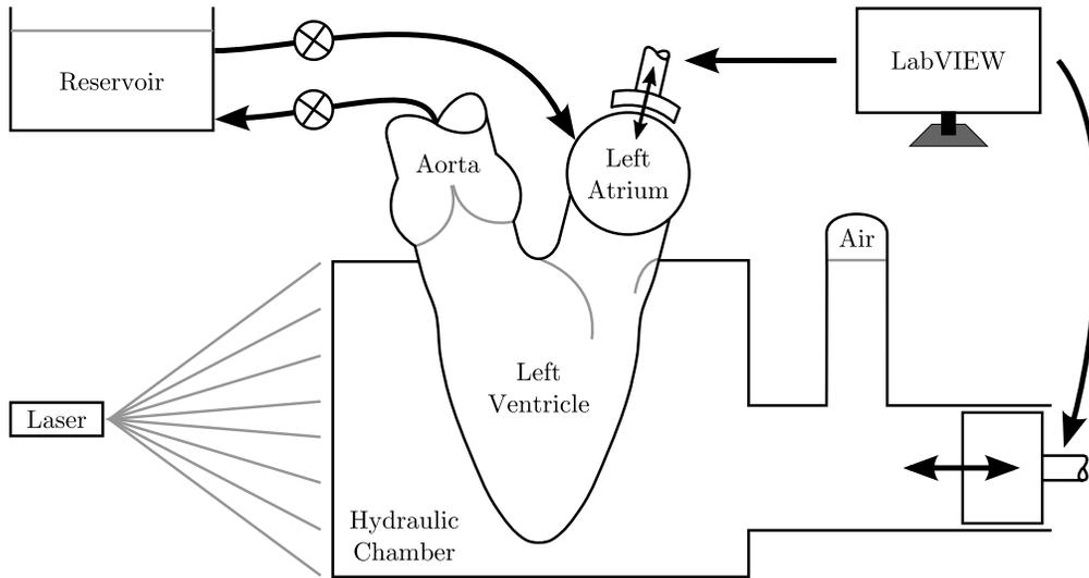
Figure 3: Schematic of the left heart duplicator. As the piston pulls back, the left ventricle fills through the mitral valve directly from the left atrium (and reservoir). Once the piston attains its maximal backward position, the left atrium is compressed to inject additional fluid into the ventricle (*A* wave filling). This begins the piston's forward stroke, compressing the ventricle in the hydraulic chamber and ejecting fluid through the aortic valve up to the reservoir.
