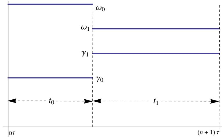
Figure 1: Krönig-Penney model for the time dependence of  $\tilde{\omega}$  and  $\gamma$  in the  $n$ - $t$  period.
