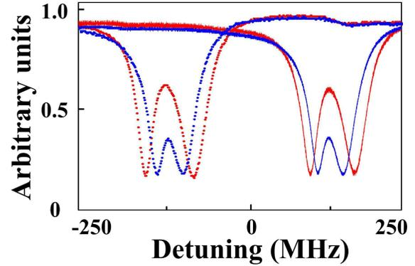
FIG. 5: (Color online). The reflective spectrum as we change the center frequency of the transparent window and the coupling strength. The coupling strength is  $\Omega = 2\pi \times 81.2$  MHz for the dark line,  $\Omega = 2\pi \times 41.8$  MHz for the gray line respectively. The center frequency of the transparent window is shifted +125 MHz for the solid line and -125 MHz for the dotted line.
