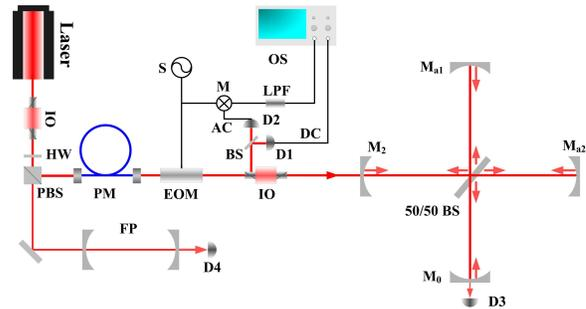
FIG. 3: (Color online). The schematic of experimental setup. IO, optical isolator; HW, half-wave plate; PBS, polarized beam splitter; PM, single-mode polarization-maintaining fiber; FP, Fabry-Pot cavity; EOM, electro-optic modulator; BS, beam splitter; S, signal generator; M, mixer; LPF, low-pass filter; D1-4, detectors; OS, oscilloscope. The power of the infrared laser before the interferometer is 10 mW.
