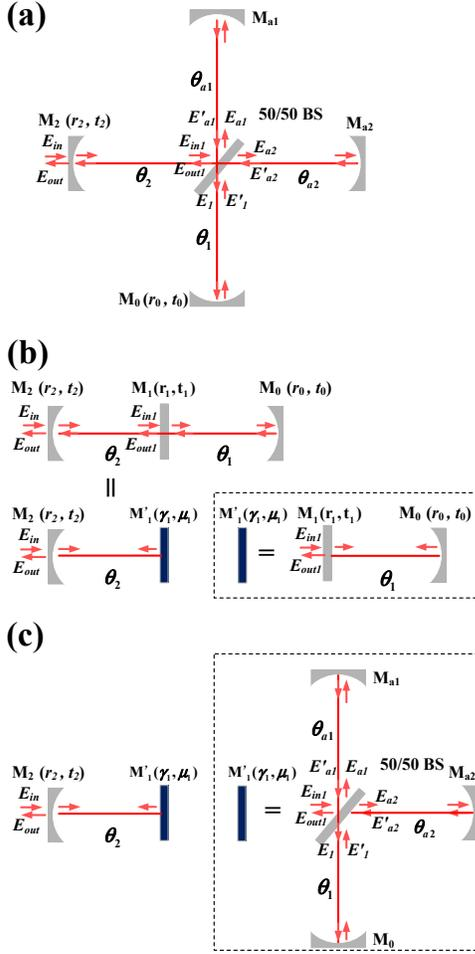
FIG. 1: (Color online). (a) The schematic diagram of dual-recycled Michelson interferometer. (b) Two coupled resonators. Inside dash line box, a single cavity is regarded as a mirror. (c) The dual-recycled Michelson interferometer can be equivalent to two coupled resonators.
