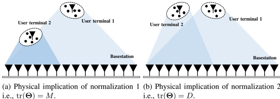
Fig. 1: Physical implication of normalization 1 (i.e.,  $\text{tr}(\Theta) = M$ ) and normalization 2 (i.e.,  $\text{tr}(\Theta) = D$ ).
