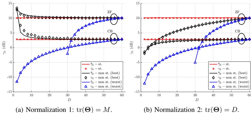
Fig. 2: The SINR vs the active number of antennas  $D$  ( $M = 60$ ,  $K = 30$ , and  $\rho = 10$  dB).
