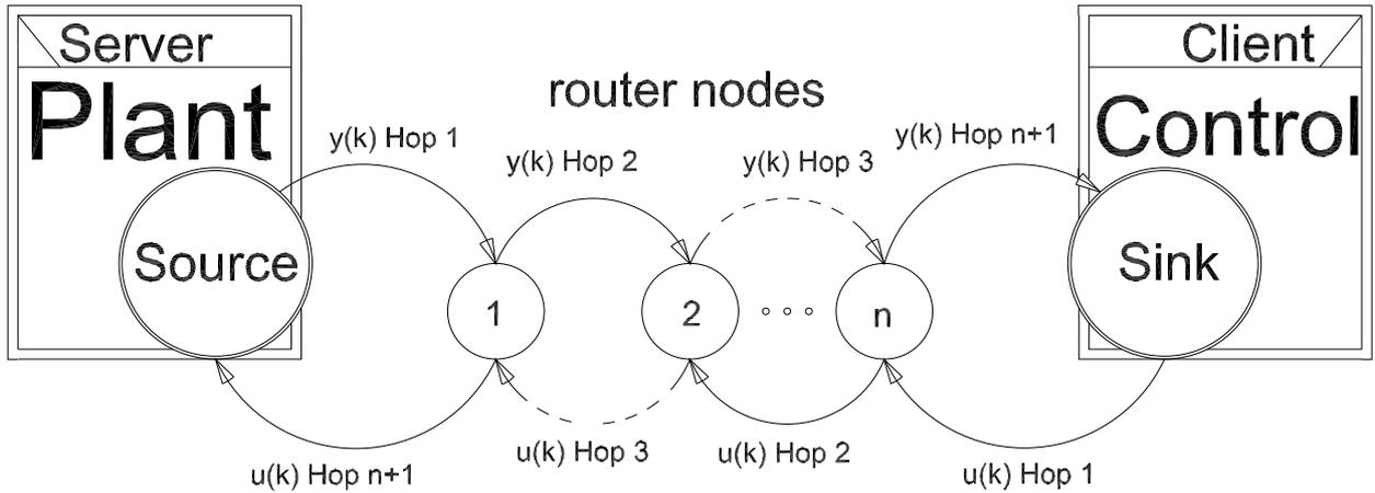
Figure 1: Control in Multi-Hop network.
