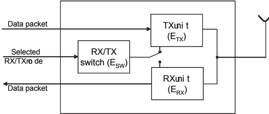
Figure 2: Energy model of radio transceiver.
