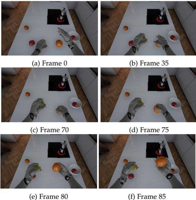
Fig. 8: Sequence of 6 frames ( $Seq = F_0, F_{35}, F_{70}, F_{75}, F_{80}, F_{85}$ ) representing a grasping action with right hand meanwhile holding a fruit with the left hand. Frames are left-right and top-down ordered
