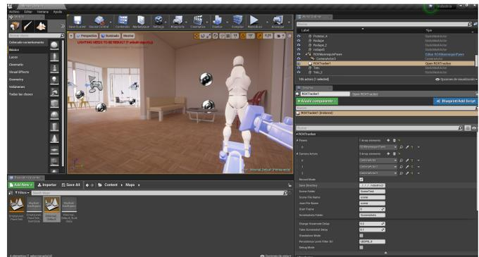
Fig. 10: *ROXTracker* custom interface showing the robot mannequin, multiple cameras, and various parameters to configure which pawns and cameras are tracked and other sequence details.
