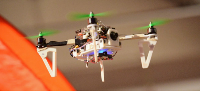
Fig. 5: Our platform, equipped with an Intel UpBoard and a Qualcomm Snapdragon Flight.
