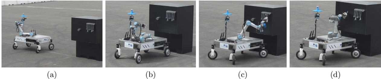
Figure 11: Our very successful second Challenge 2 run. (a) Driving around the panel to the front side; (b) Close approach; (c) Grasping the correct wrench; (d) Inserting the wrench and turning the valve.
