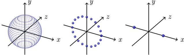
Fig. 2: Ideal simplified voting situations. *Left*: All points are uniformly distributed on a sphere ( $D = 3$ ); *Middle*: All points are uniformly distributed on a circle lying in the  $xy$  plane ( $D = 2$ ); *Right*: All points are uniformly distributed on the extremities of a segment along the  $x$  axis ( $D = 1$ ).
