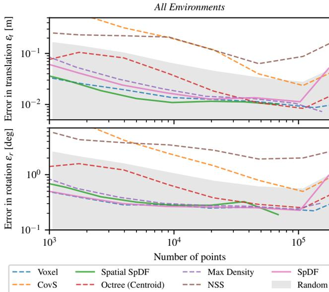
Fig. 4: Influence of the number of points on the registration process. The gray area represents the errors inferior to the baseline. Our methods are displayed in solid-line. *Top*: error in translation  $\varepsilon_t$  in m; *Bottom*: error in rotation  $\varepsilon_r$  in deg. Both translation and rotational errors show the same patterns.
