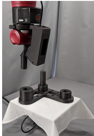
Fig. 1: Peg insertion task (0.5 mm clearance).
