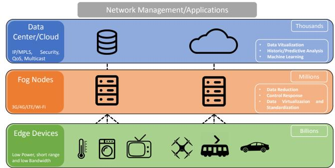
Fig. 2. High-level description of distributed EC architecture.
