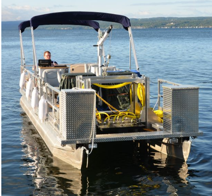
FIGURE 1. The test platform is a nine-meter pontoon boat. The projector and receive array are shown here mounted in the forward portion of the boat. These components are mounted in a rectangular frame that is lowered into the water during testing.
