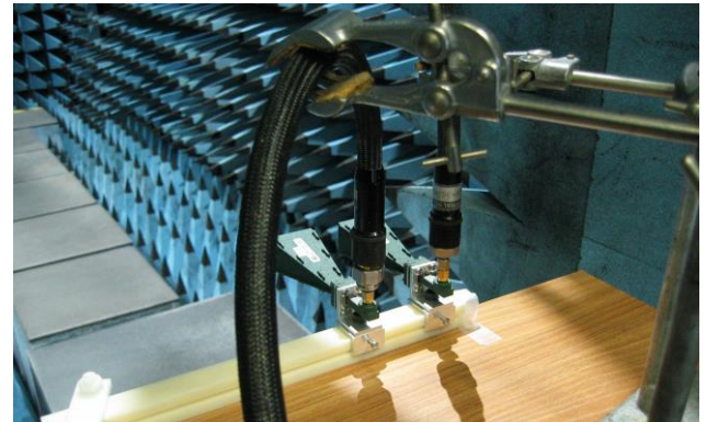
Figure 8. Experimental setup for the antenna coupling measurements in anechoic chamber at NPL.
