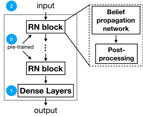
Figure 3: Structure of the entire network, and the training order labeled by the blue circles. After loading the pre-trained belief propagation network into RN block, the first step is to train the dense layers, and the second step is to train all the layers together. We will call the second step global training.
