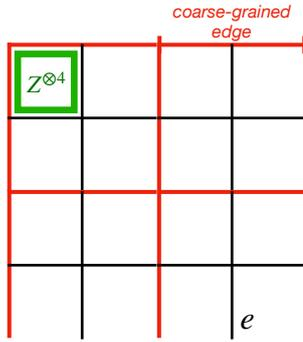
Figure 1: An illustration of the lattice and a  $B_p$  stabilizer check. The  $2 \times 2$  unit cells are marked by the red color. We also give an example of a coarse-grained edge, which locates at the top-right and contains two edges of the original lattice.
