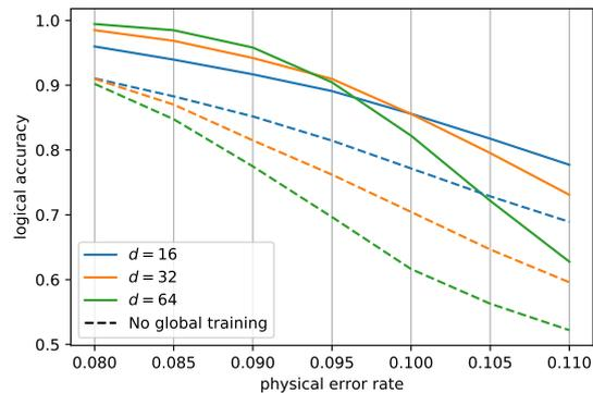
Figure 4: Logical accuracy versus physical error rate. The neural decoders are trained at physical error rate 9%. For the three solid lines, the decoder has been trained globally, while the dashed lines it has not. The colors of the dashed lines indicate the code distance they are evaluated on. The vertical grid indicates the physical error rates for which we evaluate the logical accuracy.
